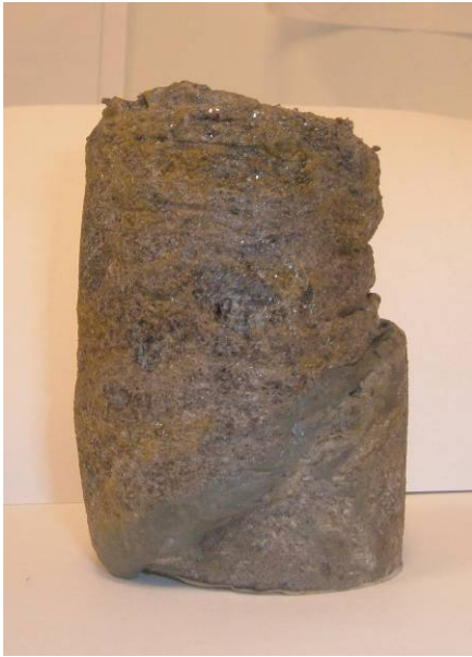
Figure 4-62: Sample #5 after Loading to 70% Stress Level
