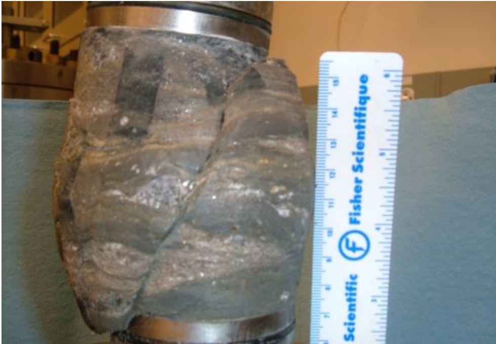
Figure 4-53: Sample #2 after Failure
