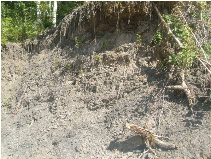
Figure 5-60: Another Exposure of the North Slope Toe showing Some Stratified Sediments
