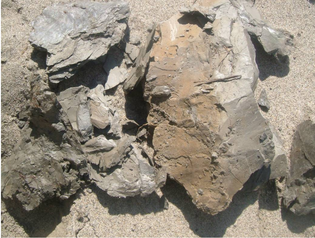
Figure 5-61: Block Samples of Sub-till Clays Obtained from an Exposure of the North Slope Toe. Varves Not Visible
