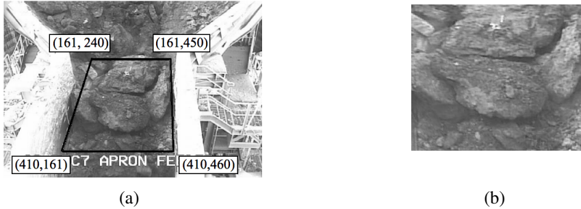
Figure 5.1: (a) An input LLD image with ROI specified by black lines. (b) ROI cut from (a) and stretched into a rectangle.
