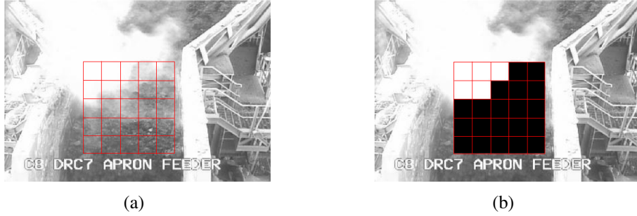
Figure 4.4: (a) An example frame from a sequence of images monitoring the dry feed preparation stage which crushes ore material in oil sands mining industry. A region of interest is selected in the image and divided into patches for steam classification. (b) The steam classification result of the input image in Fig. 4.4(a).
