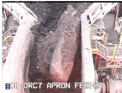
Figure 1.2: A large lump on an apron feeder before it falls into a crusher.
