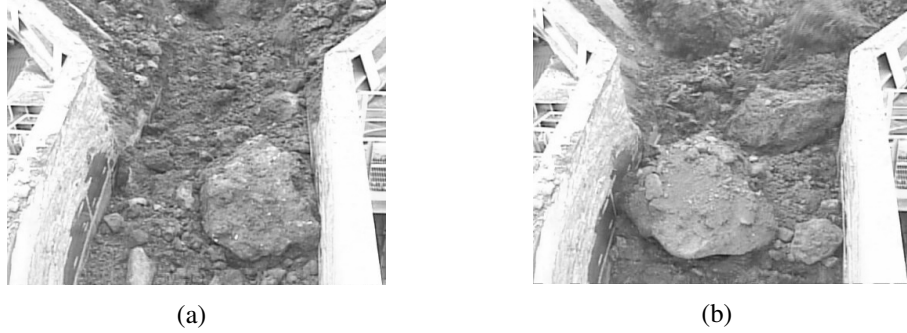
Figure 3.16: Two examples of lumps which are detected by the shape aided JDT method but not by the region based JDT method.
