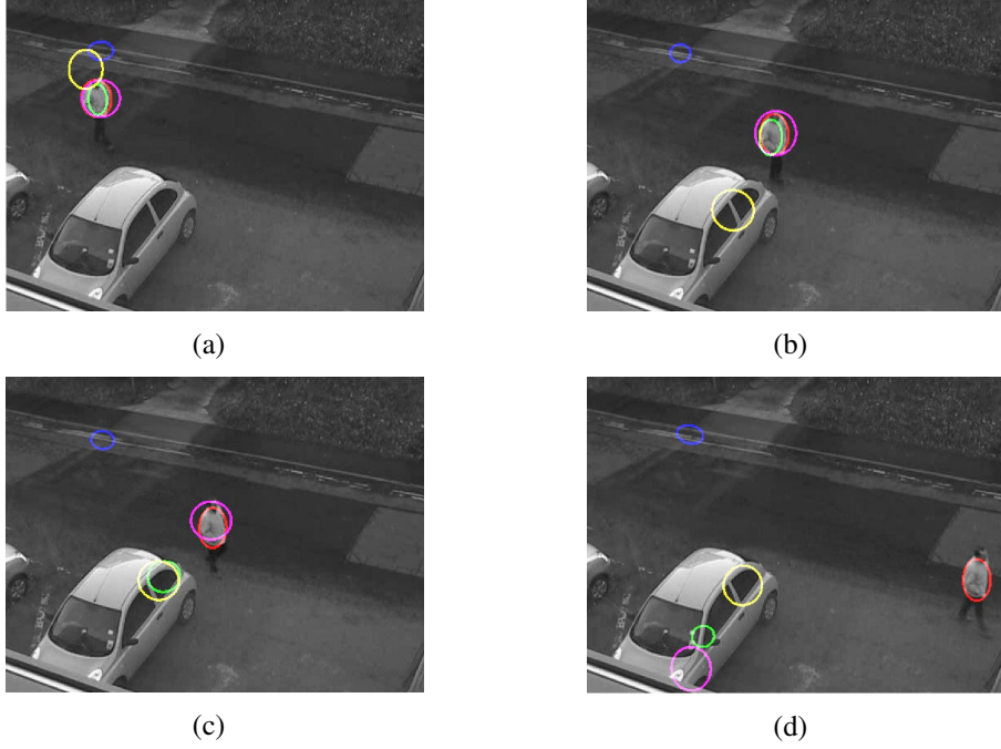
Figure 3.12: A sample of the results by the competing trackers with pedestrian sequence. (a) Frame 62. (b) Frame 113. (c) Frame 123. (d) Frame 195. The red ellipse corresponding to our method is keeping track of the pedestrian over the whole sequence. The intensity histogram based tracker (magenta ellipse) loses the track and is attracted by the car area. The boundary gradients based trackers (green, blue and yellow ellipses) are attracted by the car windows and the street curb.
