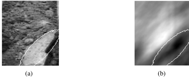
Figure 3.15: (a) A lump is described by an elliptical object state indicated by the white ellipse. (b) The average of the three square wavelet subimages computed from the original image in (a). The mean value within the object region inside the white ellipse is extracted as the smoothness feature of the corresponding object state.
