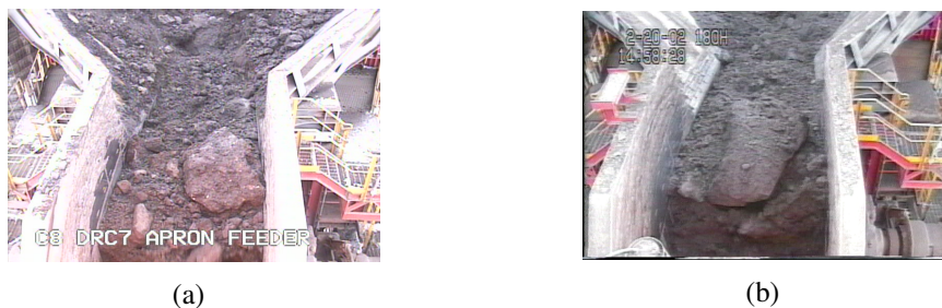
Figure 1.6: Two example images showing the similarity between the appearance of lumps and dirt.
