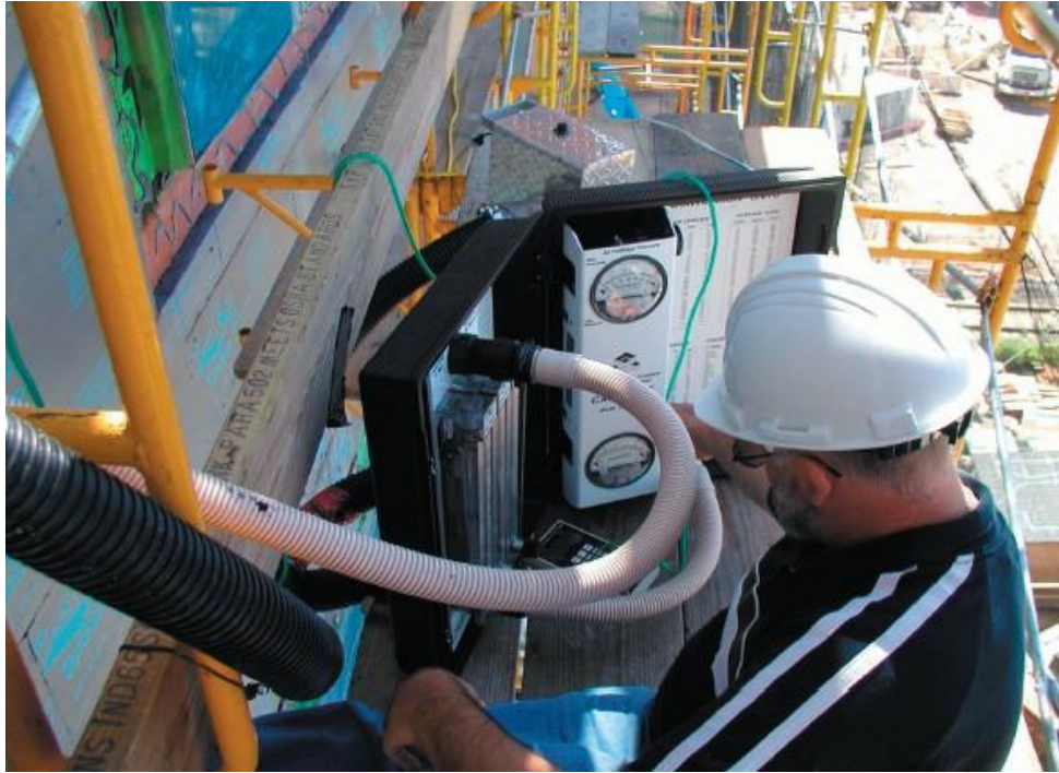
Figure 6—Airtightness test conducted by ASTM E 783(Knight and Boyle, 2010)
