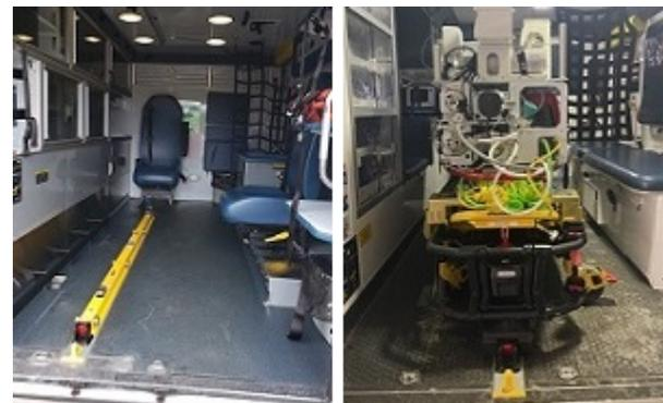
Figure 1. CHEO in Ottawa has Power-LOAD rail offset to the driver's side of the ambulance (left), while Toronto's SickKids Hospital uses a more centred rail location (right).
