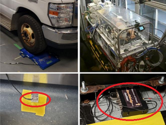
Figure 2. Test Setup - CG weighing (top-left), NPTS during road test (top-right), SPEEDBOX (bottom-right), Uni-axial floor accelerometer (bottom-left).
