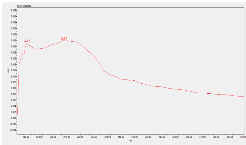
Figure 3-8- Extracted UV spectra at retention time about 8.67 minutes in HPLC analysis of reference solution diluted in chloroform
