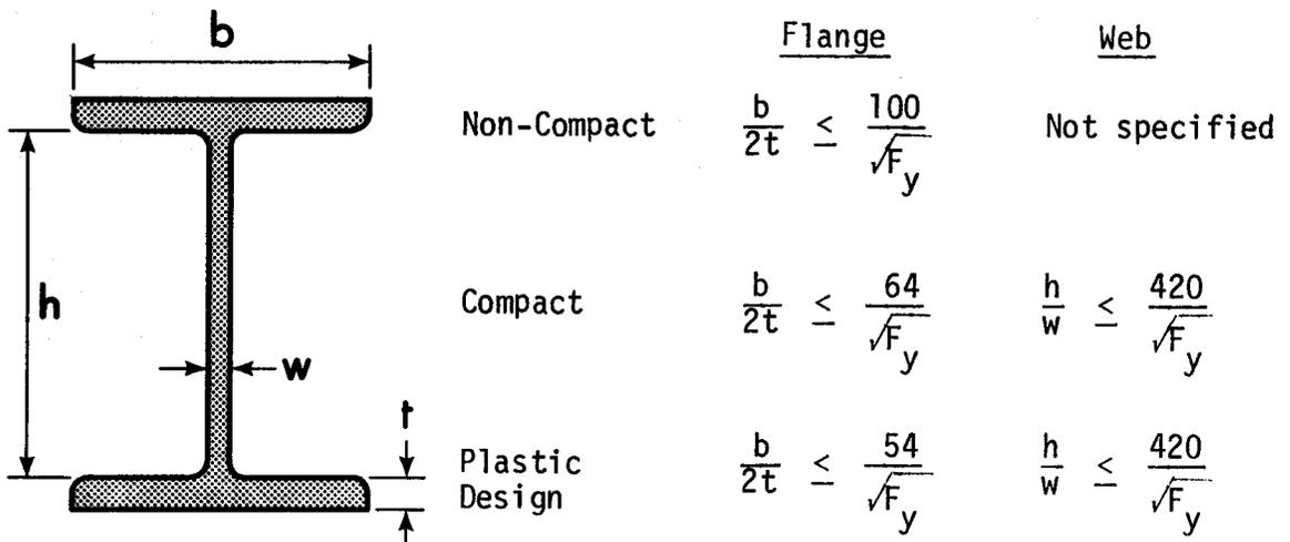
FIG. 1.2 PRESENT CSA S16 WIDTH-THICKNESS LIMITS
