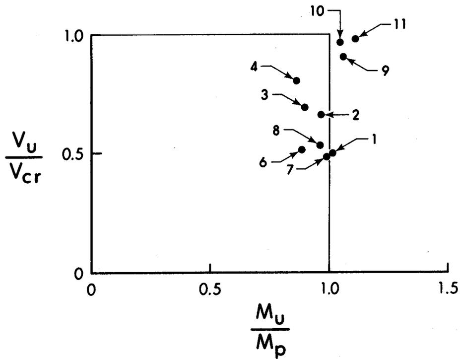
FIG. 4.2 INTERACTION OF SHEAR AND MOMENT
