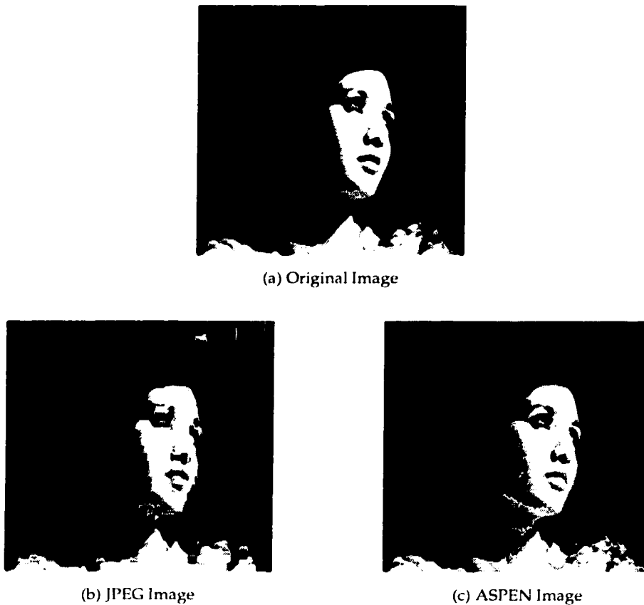
Figure 6.1: Blockiness in JPEG at low compression levels
