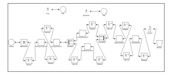
Figure 4-6: Modified simulation model to improve micro-trenching productivity
