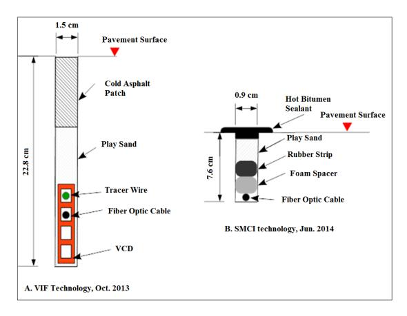
Figure 3-3: Cross section of VIF and SMCI installations
