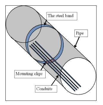
Figure 2-4: SAM Installation Components. Diagram is upside down for clarity
