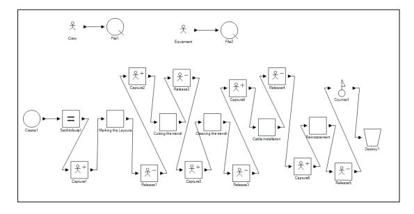
Figure 4-4: Simulation model for micro-trenching productivity analysis
