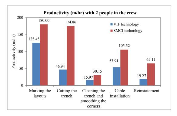
Figure 3-4: Productivity rates in both FO installation technologies
