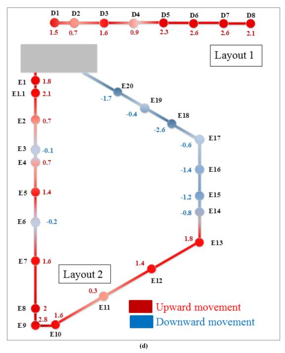
Figure 3-9: Conduit location variation relative to surface for SMCI technology- July 2014 to May 2015 (winter)
