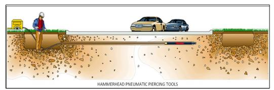
Figure 2-3: Piercing process (Reprinted from Hammerhead Trenchless Equipment 2015, with permission)
