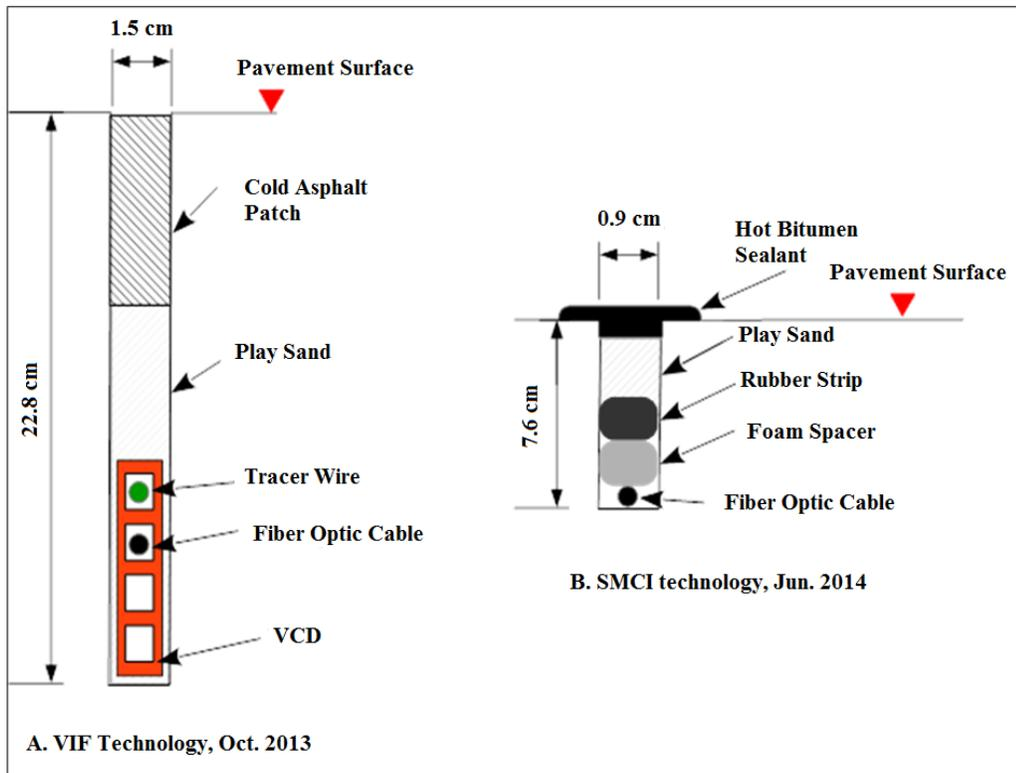
**Figure 4-3: Cross section of VIF and SMCI installations**
