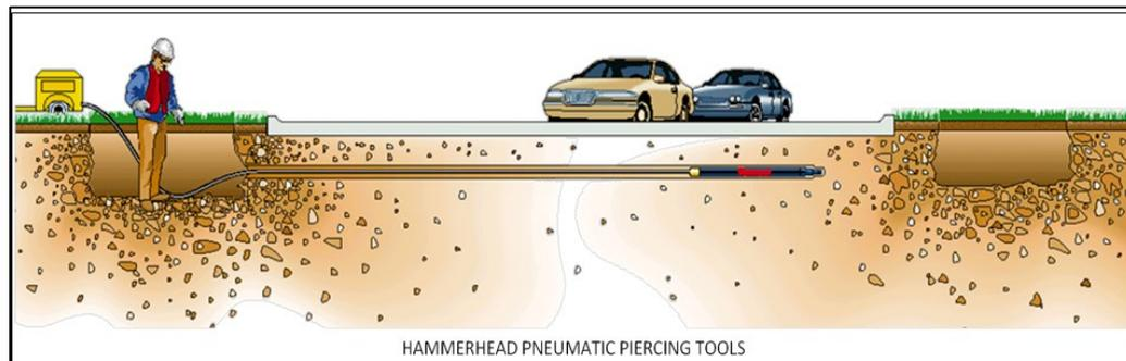
Figure 2-3: Piercing process (Reprinted from Hammerhead Trenchless Equipment 2015, with permission)
