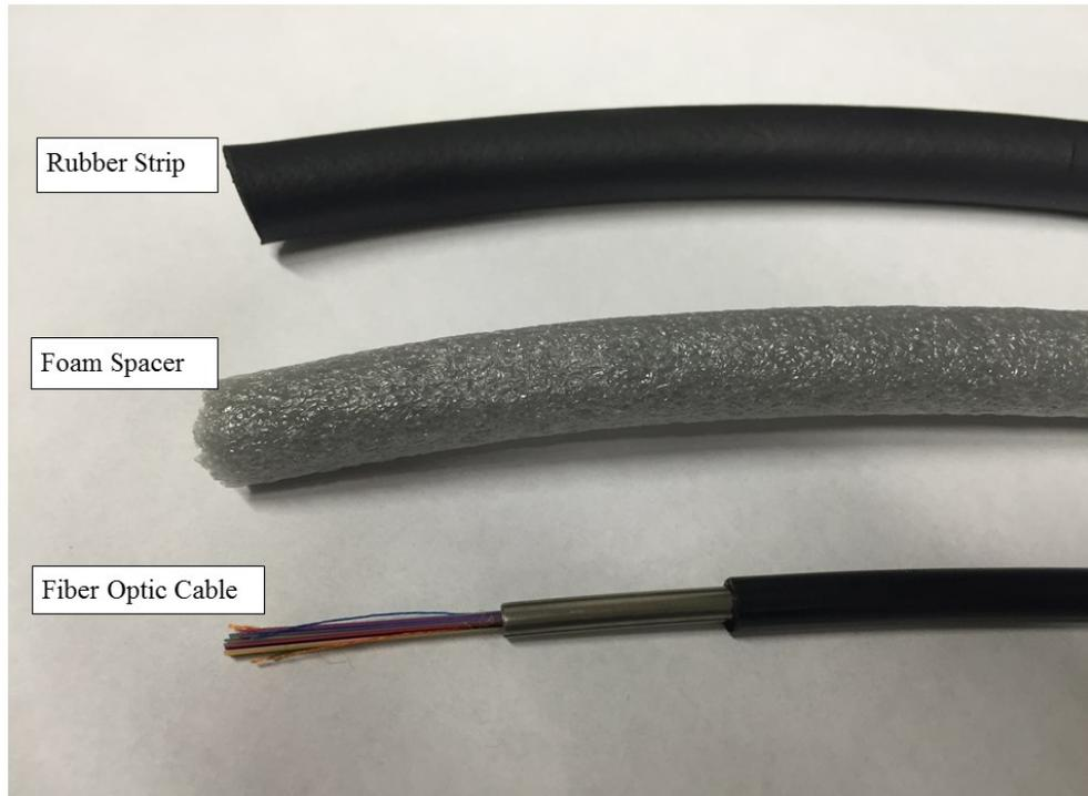
**Figure 4-2: Fiber optic cable used in SMCI**
