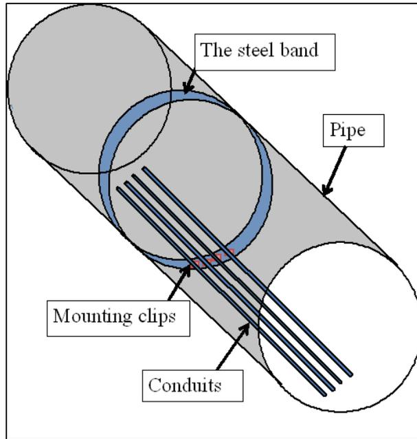
Figure 2-4: SAM Installation Components. Diagram is upside down for clarity
