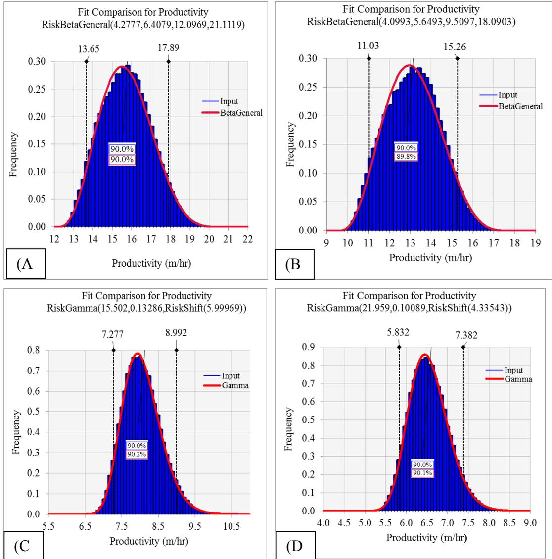
Figure 4-5: Productivity distribution: (a) Summer time, installation depth of 7.7cm, (b) Winter time, installation depth of 7.7, (c) Summer time, installation depth of 22cm, (d) Winter time, installation depth of 22cm
