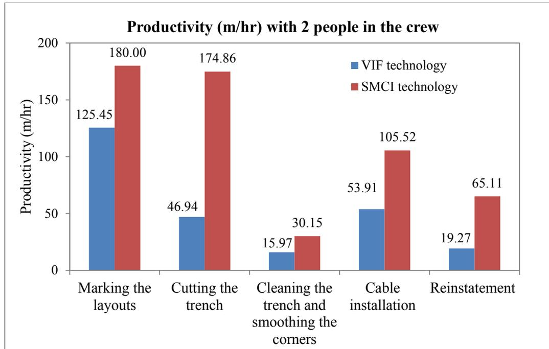
Figure 3-4: Productivity rates in both FO installation technologies
