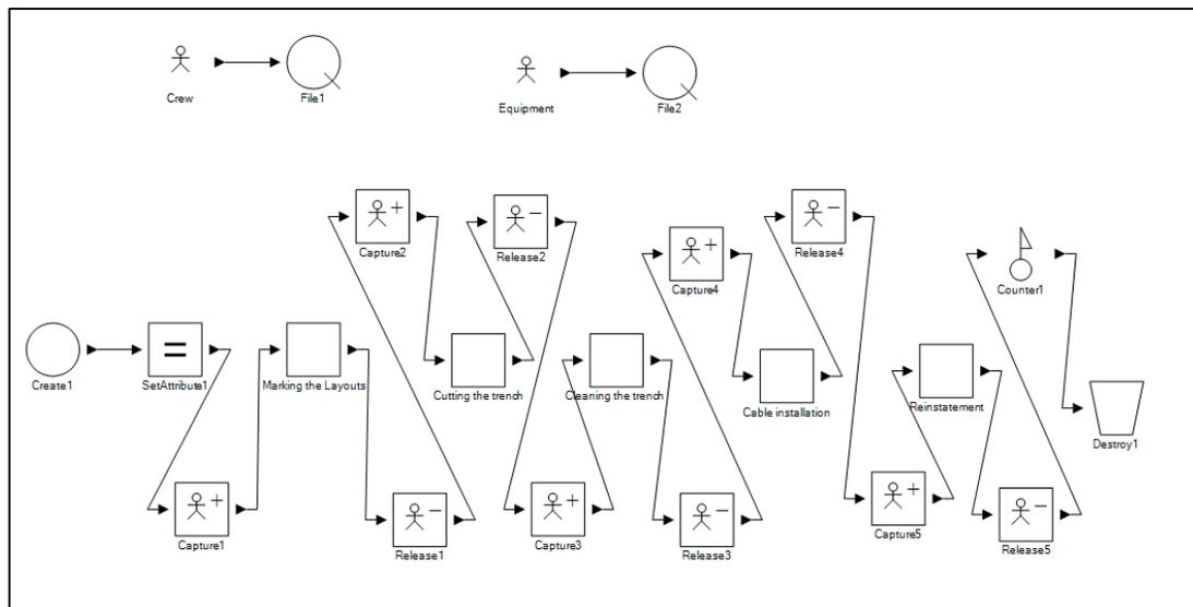
Figure 4-4: Simulation model for micro-trenching productivity analysis
