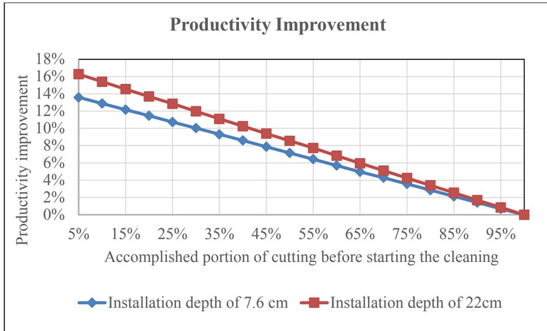
**Figure 4-7: Productivity improvement vs. completed portion of cutting before starting the cleaning**
