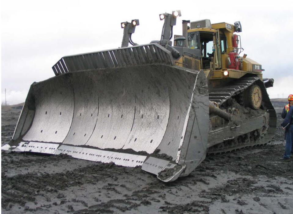
Figure 1.1: Caterpillar D11 heavy dozer in service [4].
