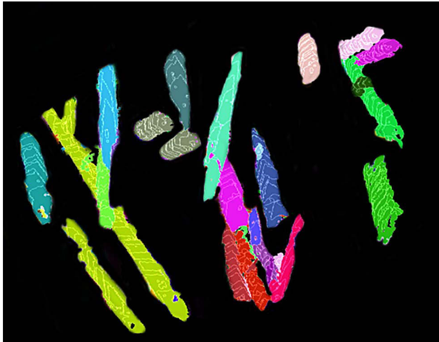
Figure 2.10: Top view of the rendered 3D reconstruction with isolated primary carbides.
