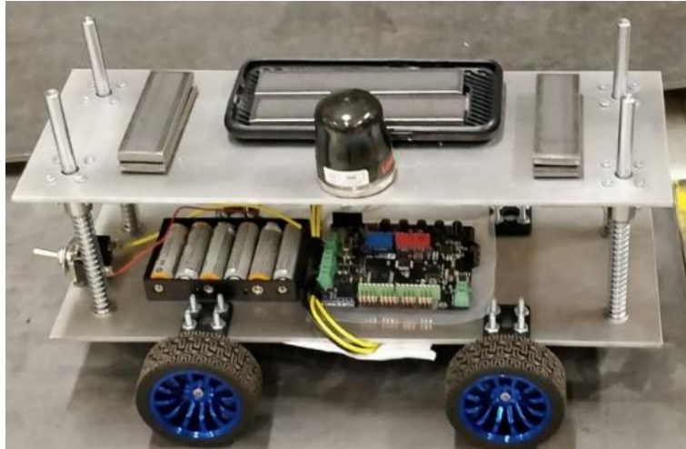
Figure 5.2 Vehicle to induce vibration in the bridge
