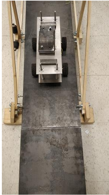
Figure 5.8 Vehicle passing over the truss bridge deck
