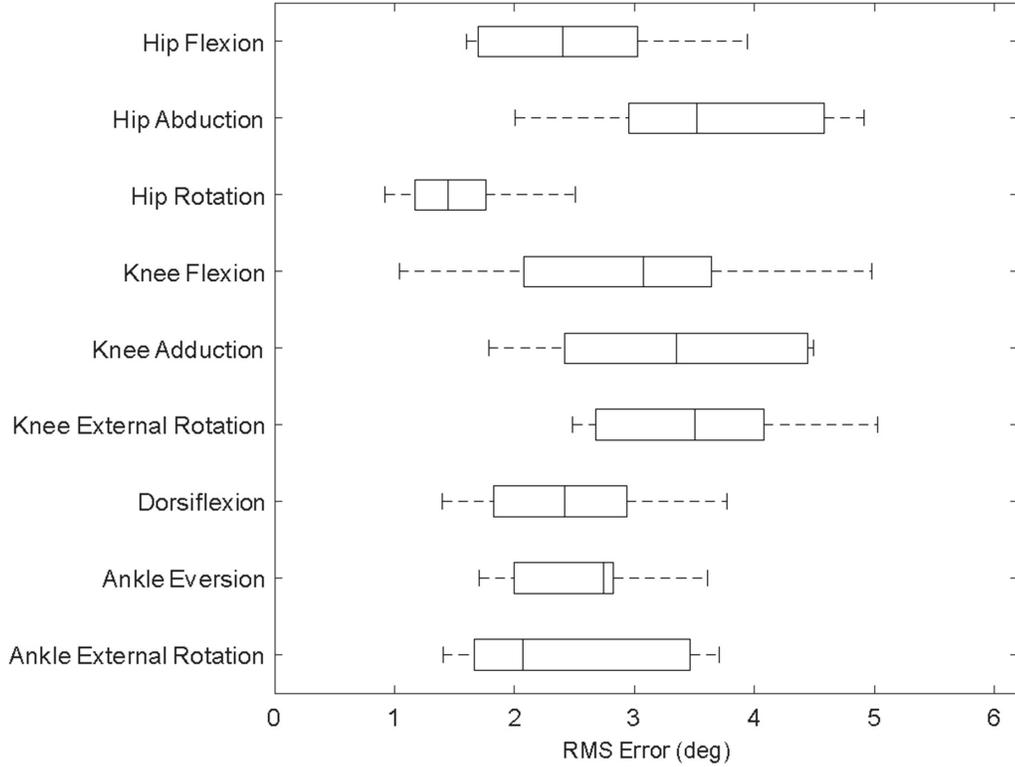
Figure 4.5: Root mean square (RMS) errors between the 3D angles obtained by IMUs readout and those obtained using camera recordings (as the reference system). First, the RMS error was attained between IMU-based and motion capture-based angles for each trial. Then, these values were averaged over all trials of each participant. Then, the RMS of all the participants' obtained average values is presented as boxplots.
