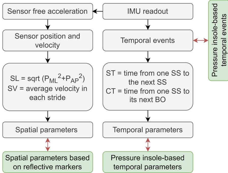
Figure 3.3: Flowchart of the measurement of temporal and spatial parameters of ice skating using IMU readouts and comparing it with the ones obtained by stationary in-lab reference systems. Here, sqrt stands for square root,  $P_{ML}$  and  $P_{AP}$ , respectively, are the travel distance in the mediolateral and anteroposterior directions in each stride.
