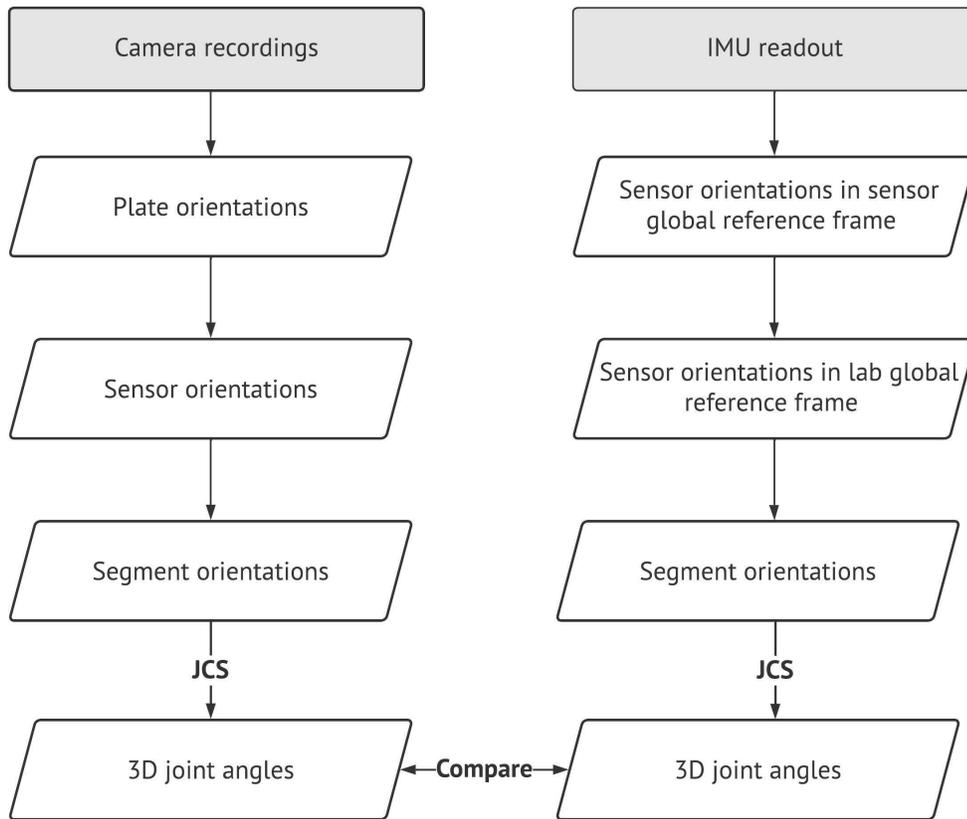
Figure 4.2: Flowchart of obtaining 3D joint angles of ice skating using IMU readouts and comparing them with the ones obtained by a stationary motion capture system.
