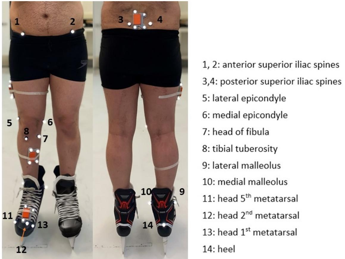
Figure 4.1: Four IMUs (orange boxes) were placed on the participants’ pelvis, shanks and skate. Also, 14 retro-reflective markers were used for 3D joint angle estimation using a motion capture system.
