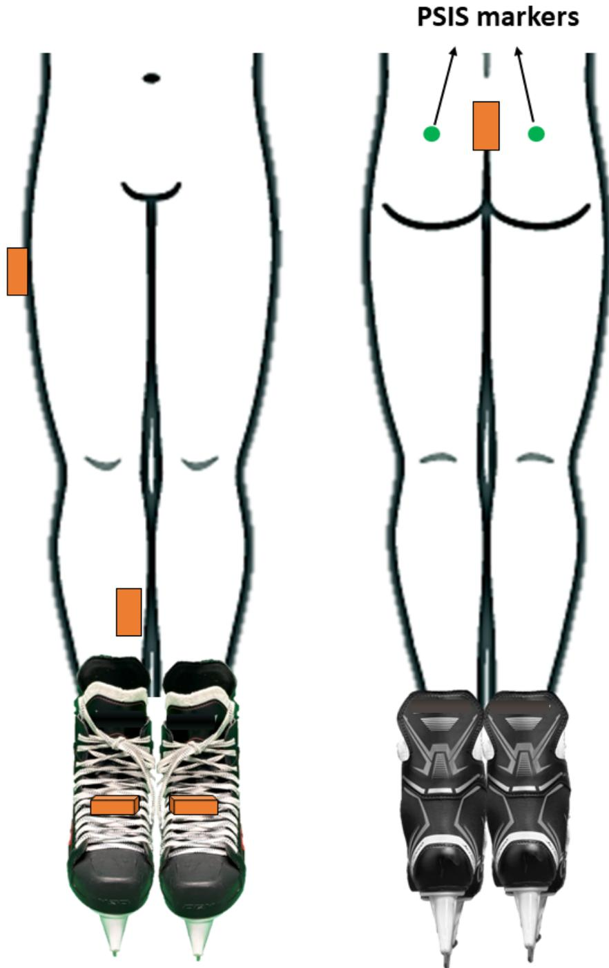
Figure 3.1: Five IMUs (orange boxes) were placed on the participants' pelvis, shanks and skates. Also, two pressure insoles placed in the skates and two retro-reflective markers on the PSISs (green circles) were used as a reference system for temporal event detection and stride length estimation, respectively.
