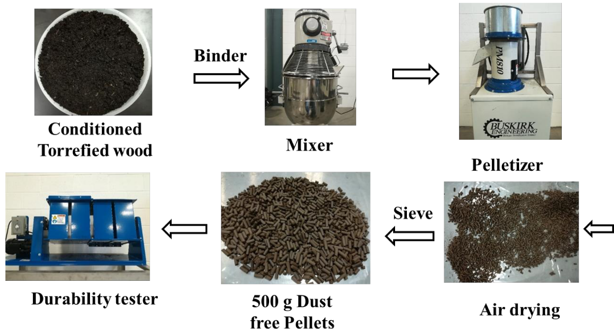
Figure 3.1. Flow chart of pilot scale pelletization and durability test
