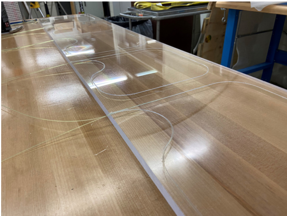
Figure 2.6: A scintillating tile prototype for testing.
