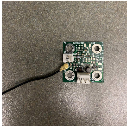
Figure 2.20: Electronic board driving the SiPM in (a).
