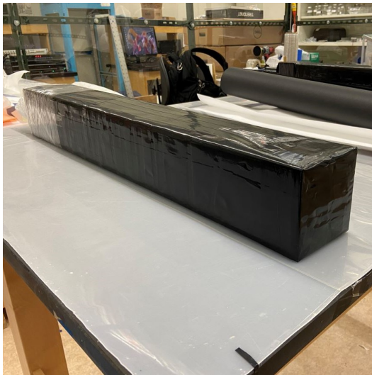
Figure 3.9: Paired scintillator bars wrapped in an effective double layer of black tape.
