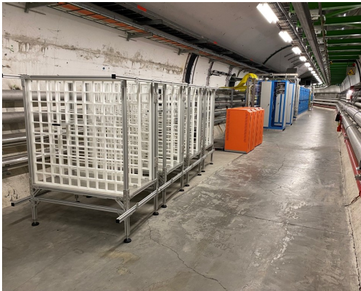
Figure 3.15: MAPP-mCP's HDPE 500 frame grids and sturdy aluminum frame.
