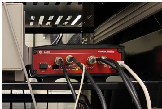
Figure 3.33: Digitizer used to send incoming PMT signals to the computer.
