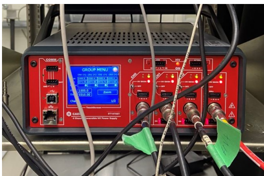
Figure 3.32: HV supply driving four channels at the same time.
