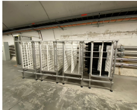
Figure 3.16: Preliminary assembly of the MAPP-mCP detector at CERN.
