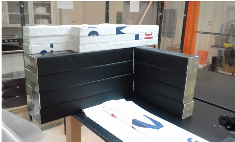
Figure 3.8: Paired bars (previously wrapped in a second Tyvek layer) wrapped in black paper.
