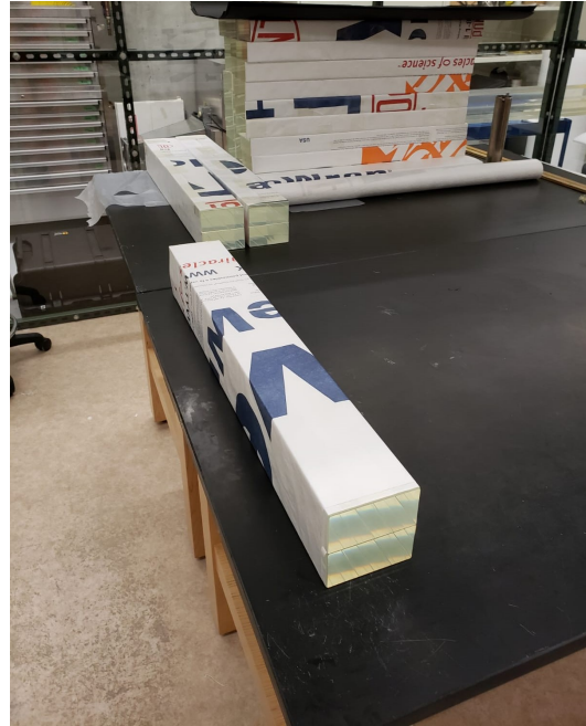
Figure 3.7: Paired scintillator bars (already wrapped in a first layer of Tyvek) wrapped in a second layer of Tyvek.
