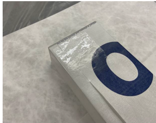
Figure 3.5: The distance between the bar's end and the end of the first Tyvek layer is of about half a centimeter.
