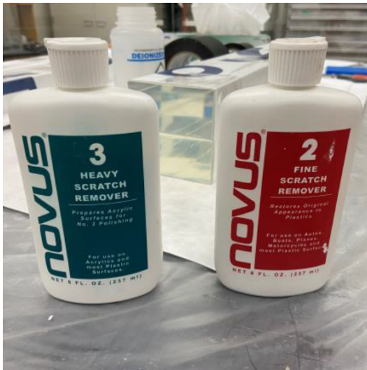
Figure 3.2: Plastic polishers used on the scintillator bars.
