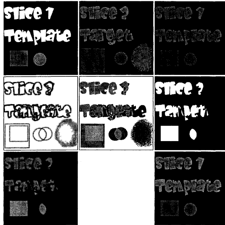
Figure 4.7: Toy example of weighting for inter-slice intensity variation reduction. The goal is to transform slice 1 so that its intensities match those of slice 2. Top row, left to right: Original slice 1, original slice 2, slice 1 scaled from unweighted linear regression. Since the objects in the two slices differ, the unweighted linear regression did not estimate a good transformation. Middle row: elements of the weighting. Left to right: Regional joint entropy, absolute difference, joint foreground pixels. Bottom left: Combined weighting (darker regions receive less weight). Note that the weighting focuses the estimation on regions that should have the same intensity. Bottom right: Linear regression using the combined weighting estimates a near-optimal linear scaling.
