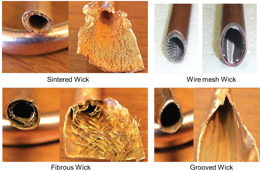
Figure 1.2: Wick types (a) Sintered wick (b) Wire mesh wick (c) Fibrous wick (d) Grooved wick. (From [50]; used with permission.)
