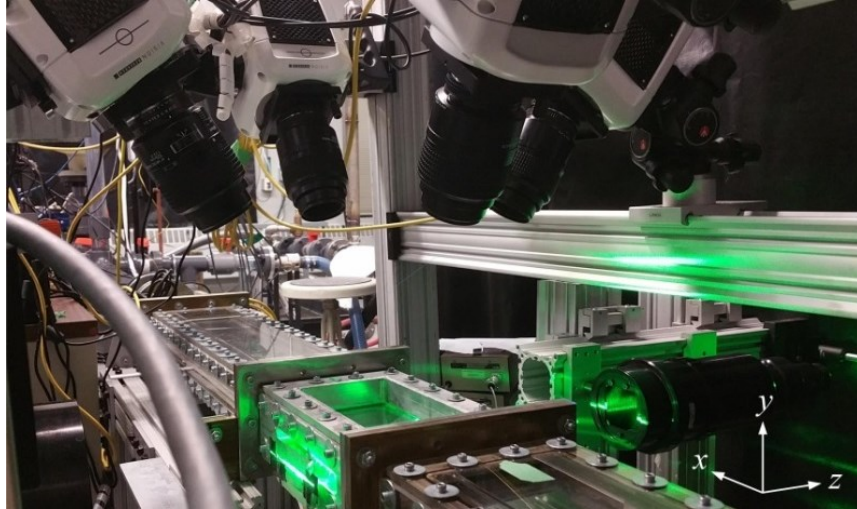
Figure 3.11. Experimental setup of 3D measurements in a symmetrical cross-like configuration with solid angle of \sim 35^\circ .
