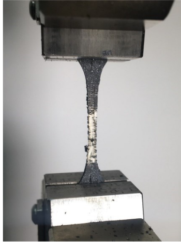
Figure 5.7. A specimen during mechanical testing.
