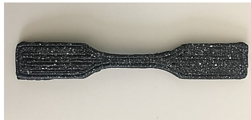
Figure 5.3. A dog-bone specimen was painted for DIC measurement.
