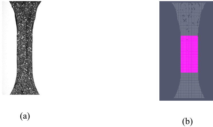
Figure 5.6. An image acquired by a high-resolution camera for DIC analysis (a) and a screenshot from Paraview software showing the area where the averaging process was applied (b).
