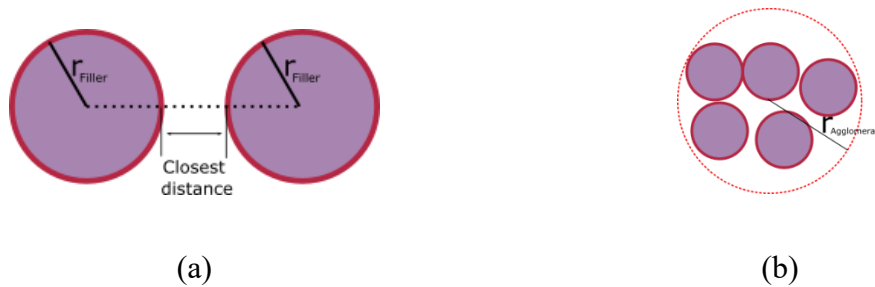
Figure 2.4. The closest distance between two fillers (a) and agglomerated fillers (b).
