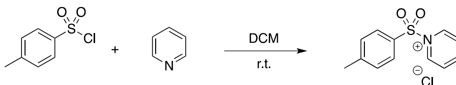
Figure 3-19. Reaction of p -Toluenesulfonyl chloride with pyridine to generate sulfonyl chloride/pyridine complex.
