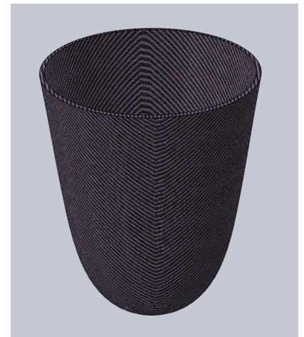
3D Model of Silicone Layer of Prosthetic Lining designed by Eric Lepp
