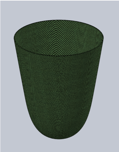
3D Model of Hemp Layer of Prosthetic Lining designed by Eric Lepp
