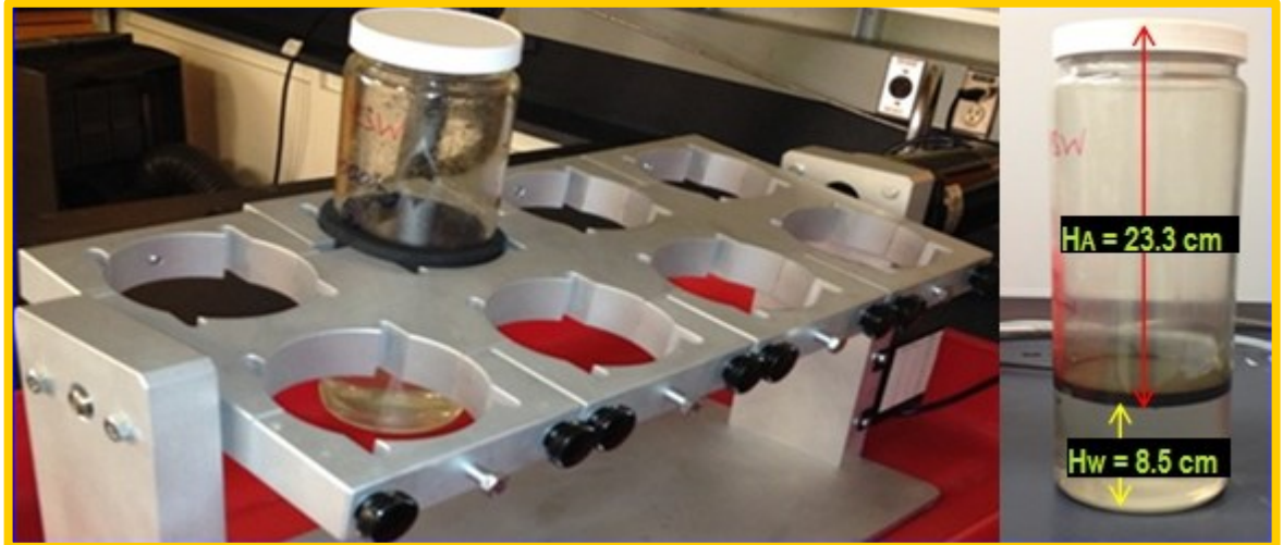
Fig. 1. Experiment setup, an orbital agitator and a jar sample
