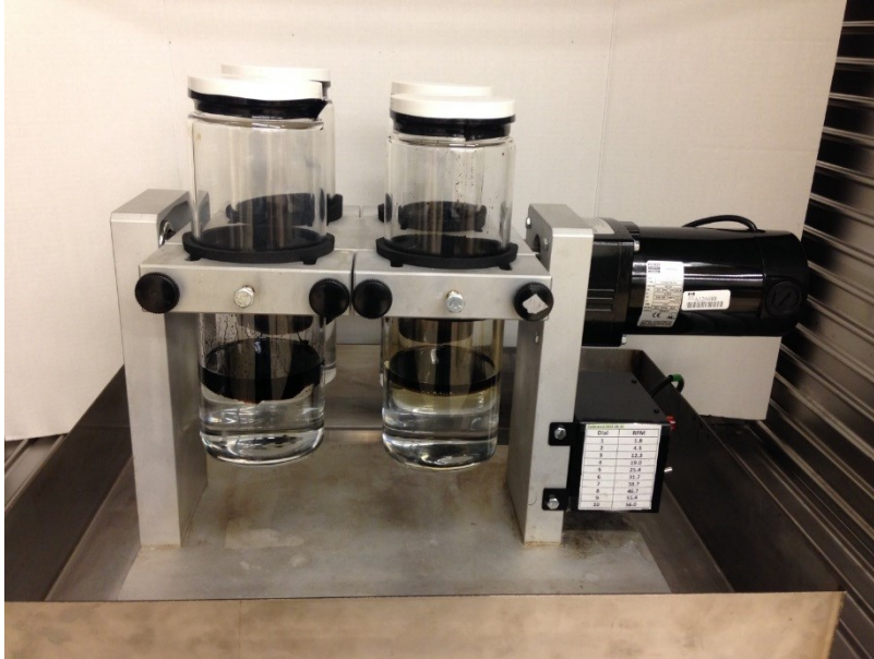
Figure 1-4: Image of the mixing jars mounted on the rotary agitator
