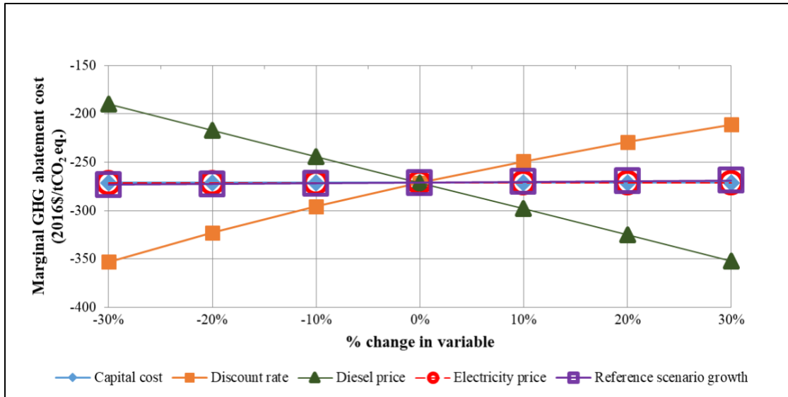
Figure A5: IR-TMS scenario sensitivity of abatement cost to capital cost, discount rate, diesel price, electricity price, and reference scenario growth
