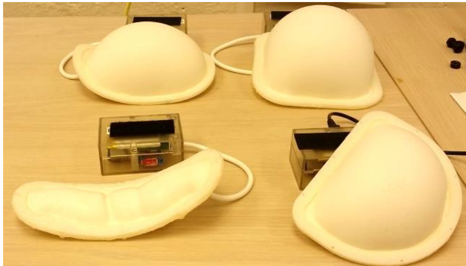
Figure 4 - 11 Manufactured dynamic brace pads. Top left: thoracic pad. Top right: trochanter pad. Bottom left: lumbar pad. Bottom right: axilla pad.
