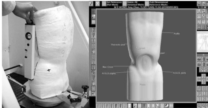
Figure 2 - 12 Brace manufacturing methods. (a) Manual method cast rectification [71]. (b) CAD/CAM method cast rectification [15].
