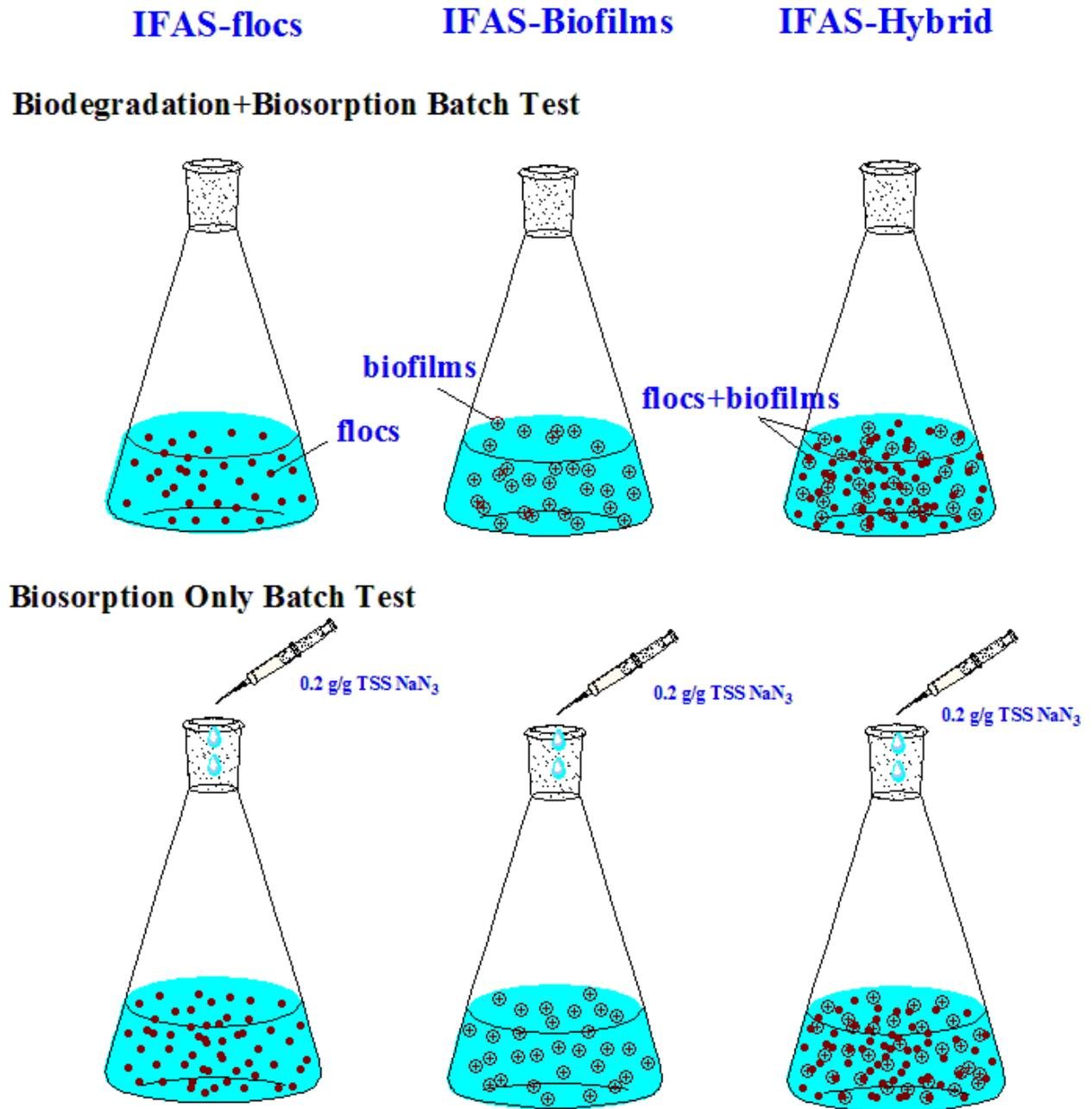
**Figure 5.1.** The schematic diagram of batch IFAS reactors.
