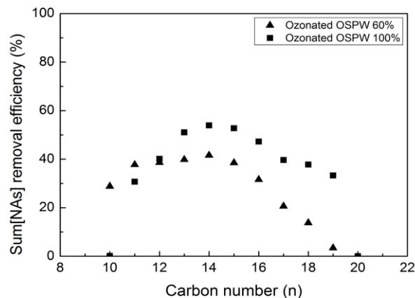
**Figure 3.2.** Profile of Sum [NAs] removal efficiency versus Z value (A) raw-OSPW IFAS, (B) ozonated-OSPW IFAS, profile of Sum [NAs] removal efficiency versus carbon number n (C) raw-OSPW IFAS, (D) ozonated-OSPW IFAS.
