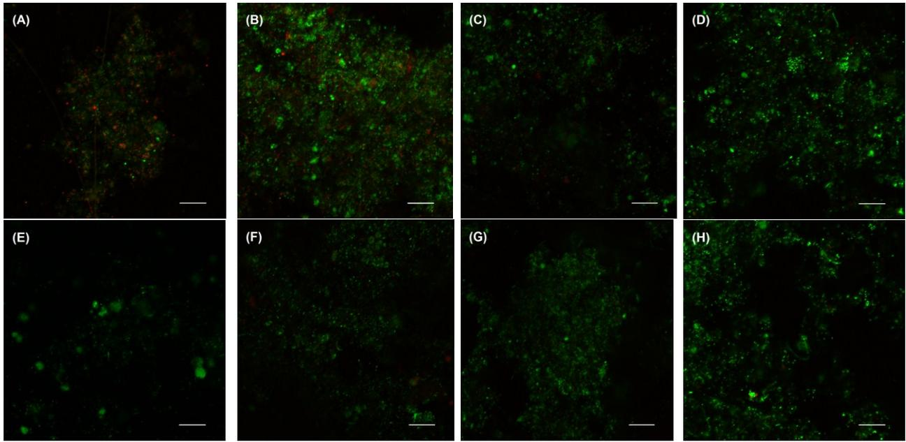
**Figure C5.** CLSM micrographs of biofilm formed on support media during the start up operation of two IFAS systems: (A), (B), (C) and (D) are the carrier cultivated for 42, 91, 130 and 161 days of raw-OSPW IFAS system; (E), (F), (G) and (H) are the carrier cultivated for 42, 91, 130 and 161 days of ozonated-OSPW IFAS system. Bar equal to 50 $\mu$ m.
