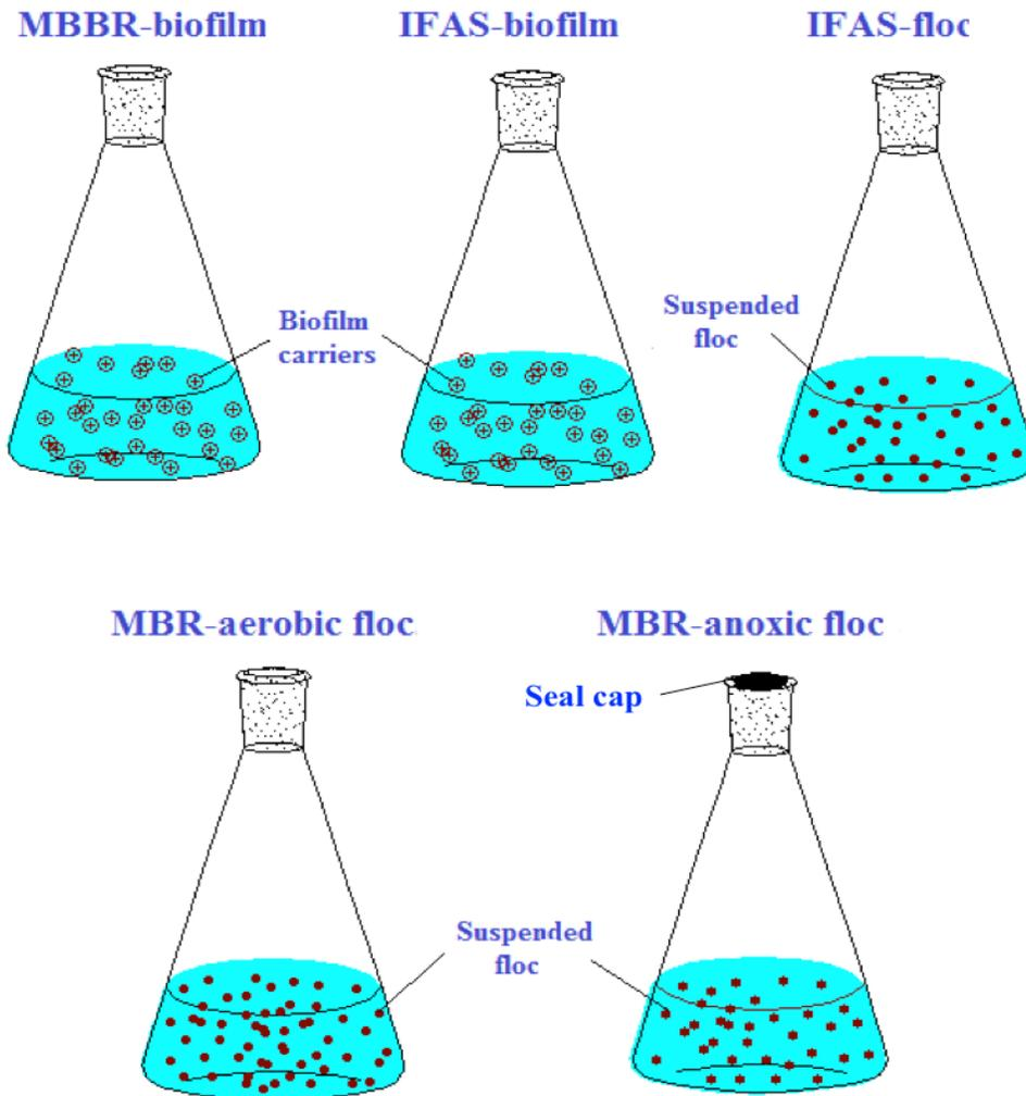
**Figure 7.1.** The schematic diagram of batch reactors
