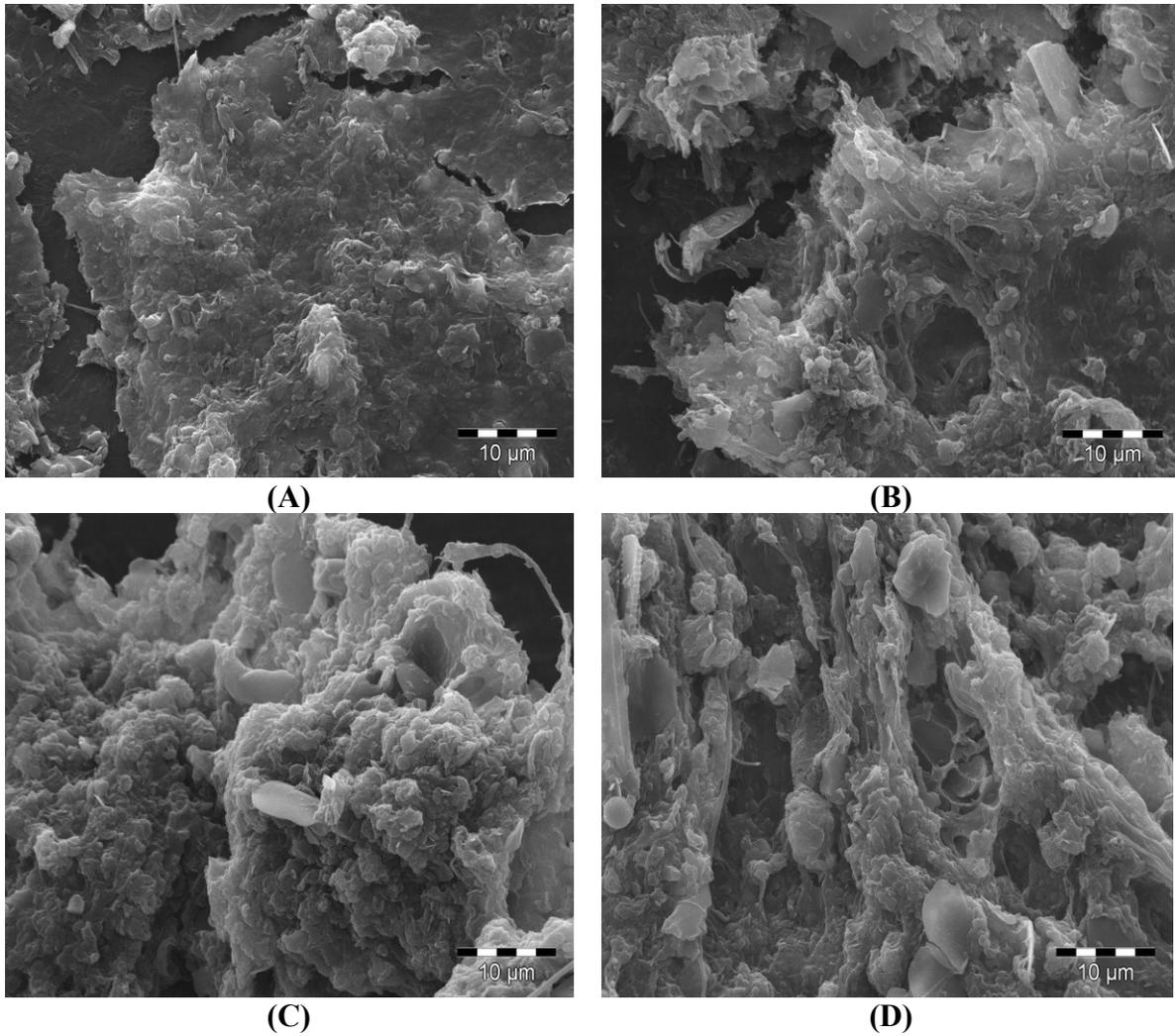
**Figure C4.** SEM micrographs of biofilm formed on biocarriers during the start up operation of two IFAS systems: (A) carrier cultivated for 82 days of raw-OSPW IFAS system; (B) carrier cultivated for 130 days raw-OSPW IFAS system; (C) carrier cultivated for 82 days of ozonated-OSPW IFAS system; (D) carrier cultivated for 130 days ozonated-OSPW IFAS system.
