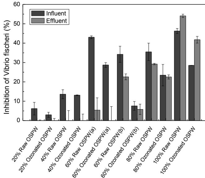
**Figure 3.4.** Toxic effects of influent and effluent of raw and ozonated-OSPW IFAS systems on *Vibrio fischeri* after 15 min of exposure at different stages.
