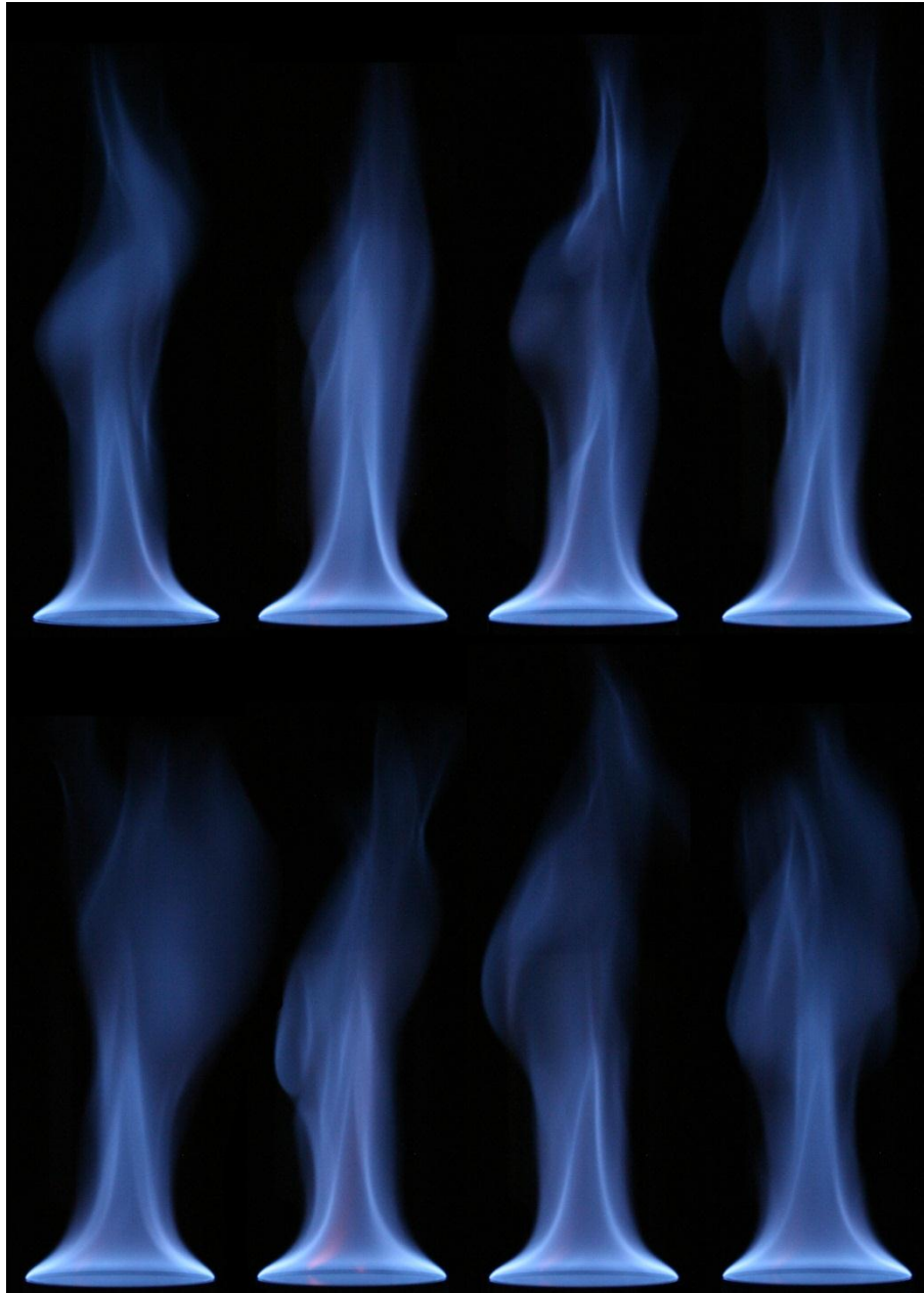
Fig. 4.6 A series of successive photographs of flame established above the methanol pool
