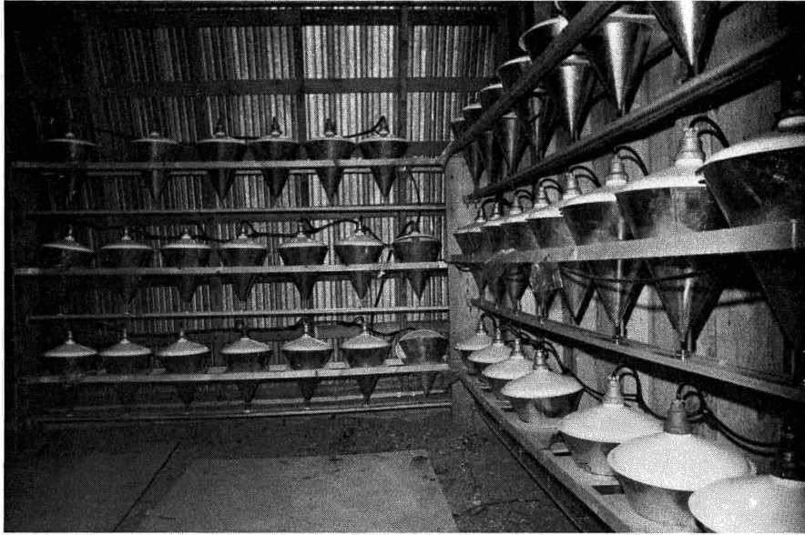
Figure 4. Set of 45 Tullgren funnels used at Mildred Lake Research Facility to extract soil insects.
