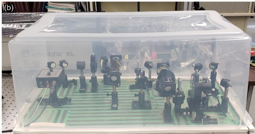
**Fig. 3.1.** (a) Schematic of the THz-TDS system typically used to conduct experimental measurements. ‘M’ indicates planar mirrors, ‘PM’ indicates parabolic mirrors, and ‘L’ indicates lenses. (b) Photograph of the THz-TDS system.
