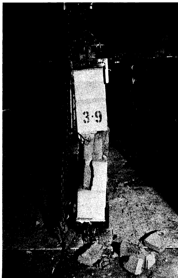
PLATE 6.7 Failure of Short Wall Specimen with 3-#9 Vertical Bars
