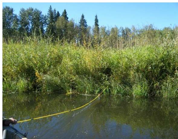
Determining the width of river and 1 meter transects for each station.
