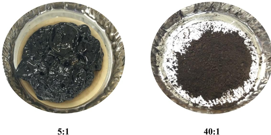
**Figure 3-5.** Appearance of C<sub>5</sub> asphaltenes precipitated at S/B ratios 5:1 and 40:1
