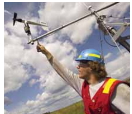
A climate station placed on an instrumented watershed measures rainfall, solar radiation, temperature, wind speed and direction, humidity and more. This information helps us determine the interaction of water, wind and heat with reclaimed landscapes.
