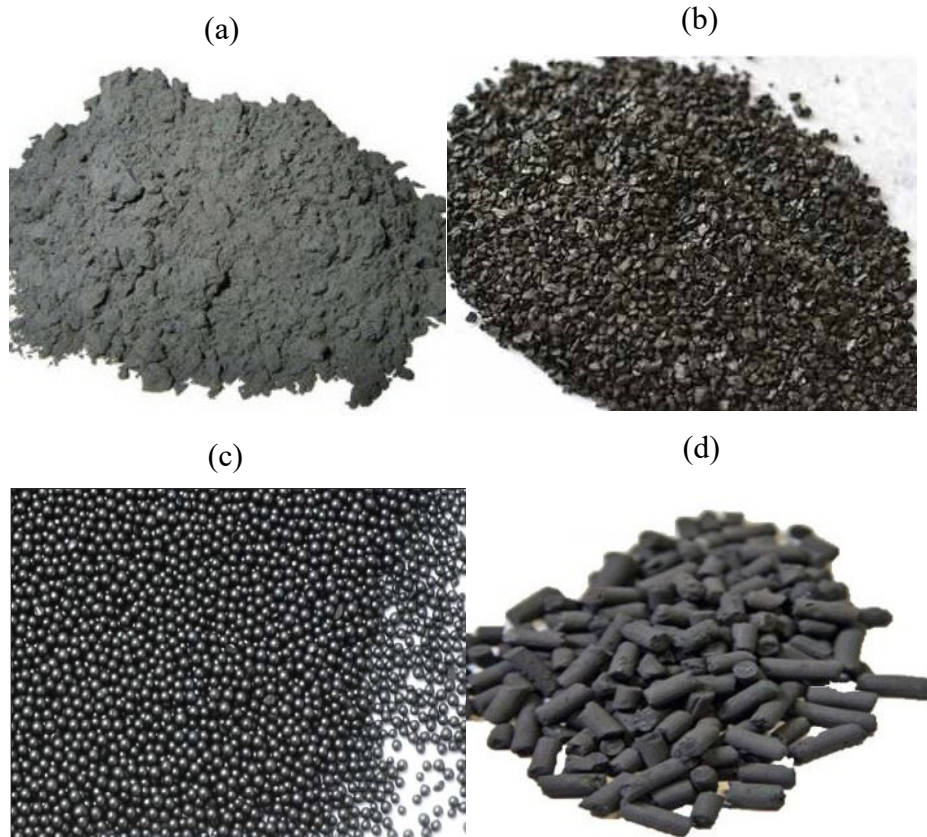
Figure 2-3. Different forms of activated carbon (a) powdered (b) granular (c) beaded (d) pelleted (Bansal and Goyal 2005)
