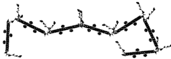
(b) Low temperature, poor solvent (linear aggregation)
