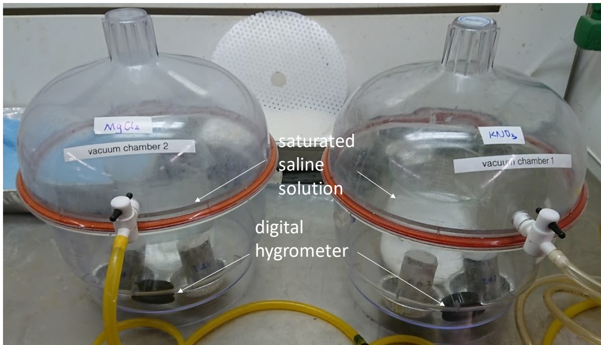
Figure 3-5. Preconditioning of the Opalinus Clay specimens under controlled total suction provided by two different saline solutions ( \text{MgCl}_2 and \text{KNO}_3 )
