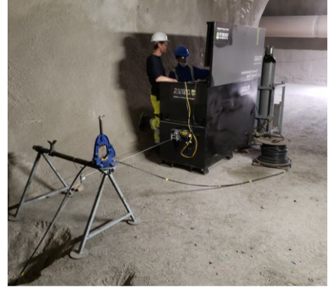
Figure A- 11. Onsite configuration for pressuremeter testing in borehole BGC-A4 (40° dipping into the floor)
