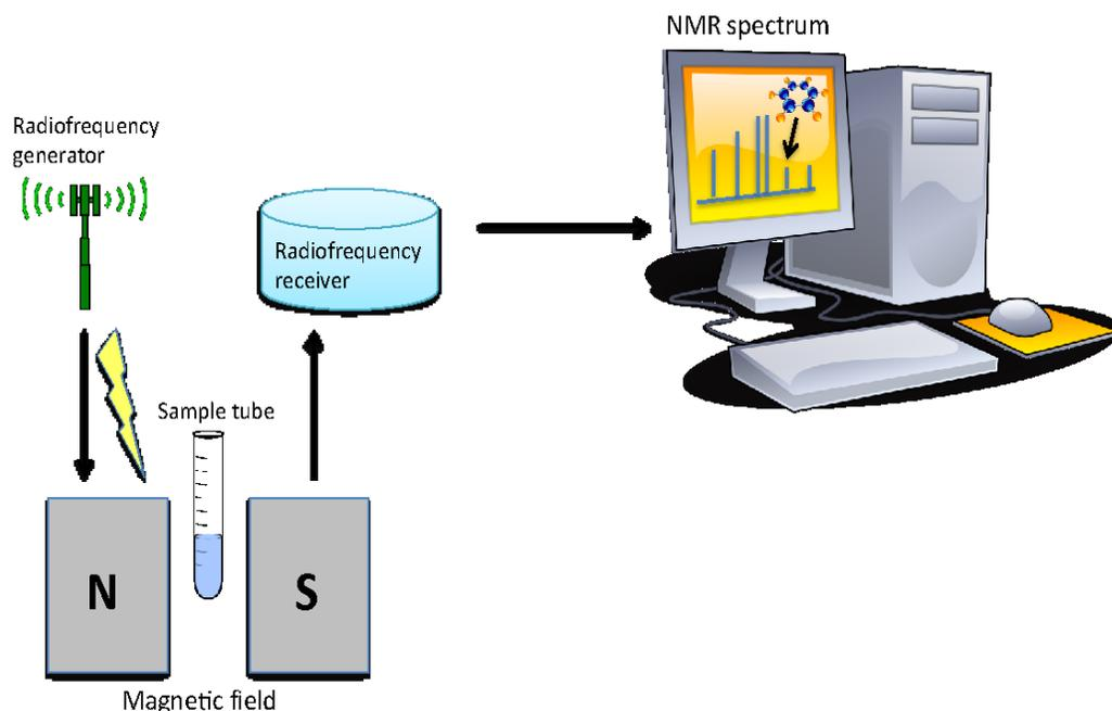
**Figure 1-2:** Schematic of NMR spectrometer.
