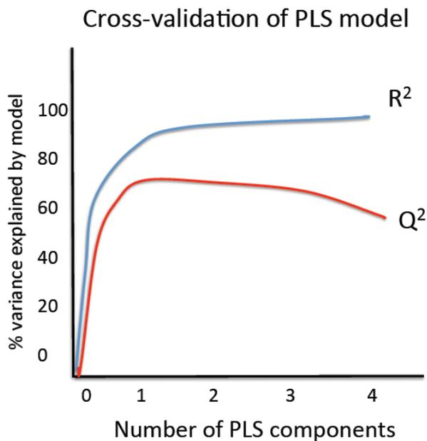
**Figure 1-4: Cross validation model.** The trade-off between the goodness of fit ( $R^2$ ) and the goodness of prediction ( $Q^2$ ). One PLS component appears to be the optimal model, as this is where maximum  $Q^2$  is seen, and difference between  $R^2$  and  $Q^2$  is reasonably small. After one PLS component, the  $Q^2$  declines indicating that the model is being fitted to noise (random error).
