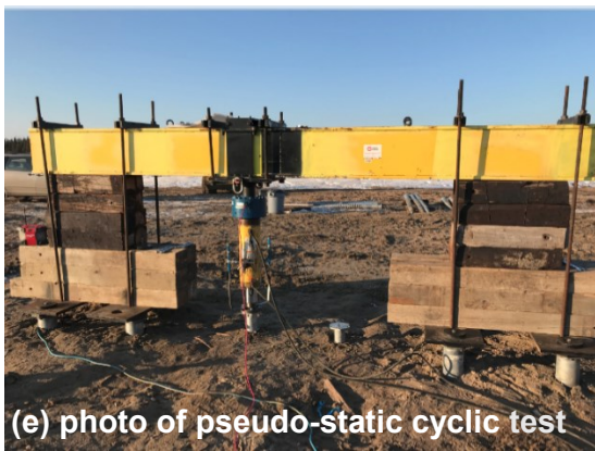
Figure 4.3. Experimental testing methods for a general SFSI study: (a) and (b) dynamic shaking test, (c) and (d) mass (or force) vibration test and (e) and (f) pseudo-static cyclic test. Note: the mass vibration and pseudo-static cyclic loading tests can also be applied in the lateral direction; (b), (d) and (f) are illustrative only and do not necessarily match the actual experimental setup.
