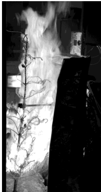
Figure 3-8: Tree burning in the radiant panel assembly
