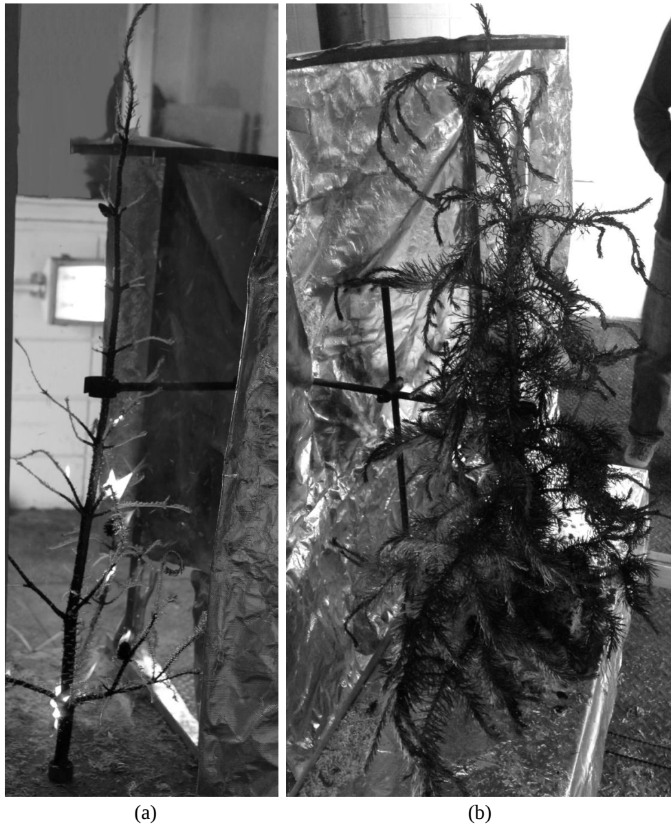
Figure 4-8: Comparison of trees after burning (a) untreated with its needles all burnt and some remnant branches and (b) treated with wet (5.5:1) long-term retardant having most of its needles and branches still intact
