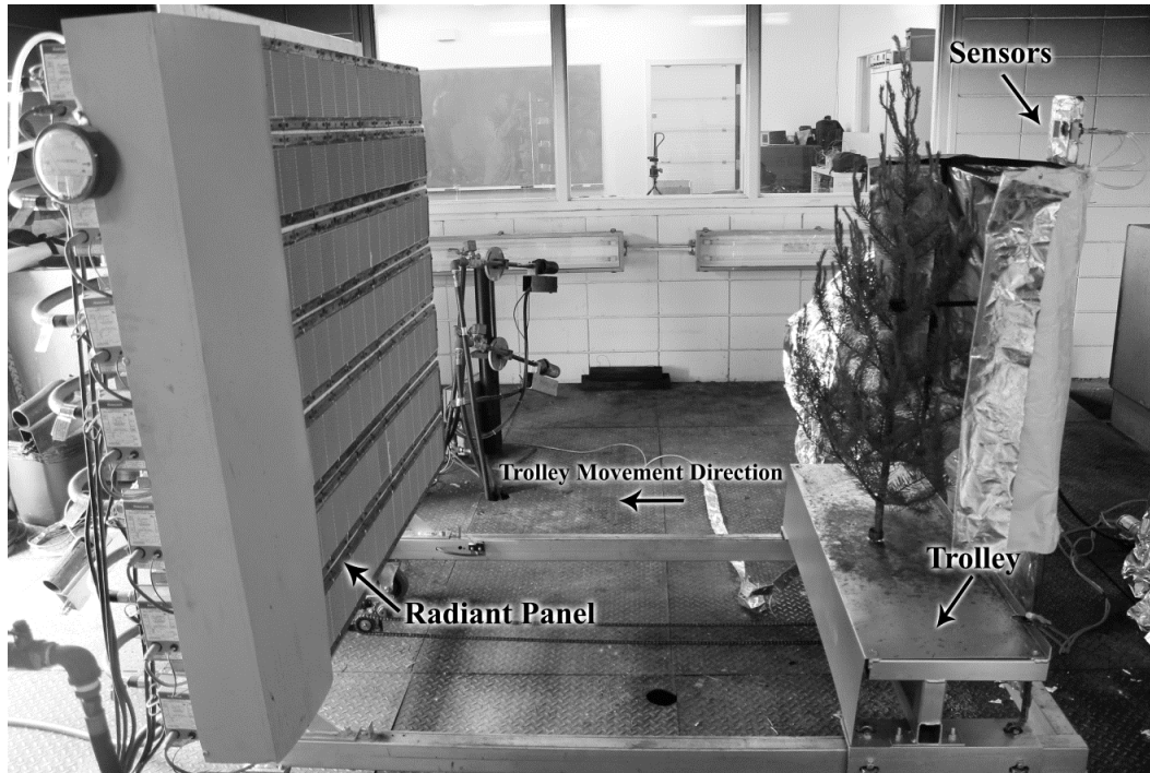
Figure 3-7: Experimental assembly for simulated fire tests
