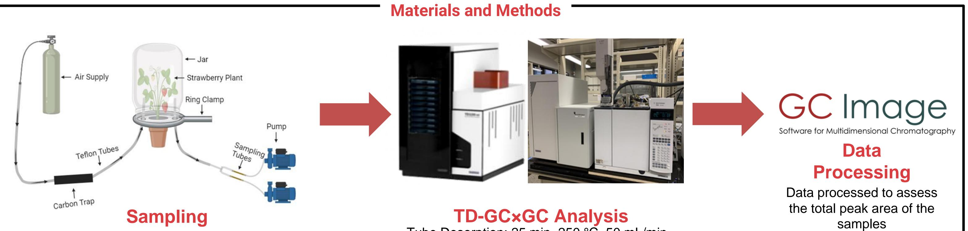
1 h Sampling Time Air Intake: 300-350 mL/min Sampling Flow Rate: 50 mL/min
