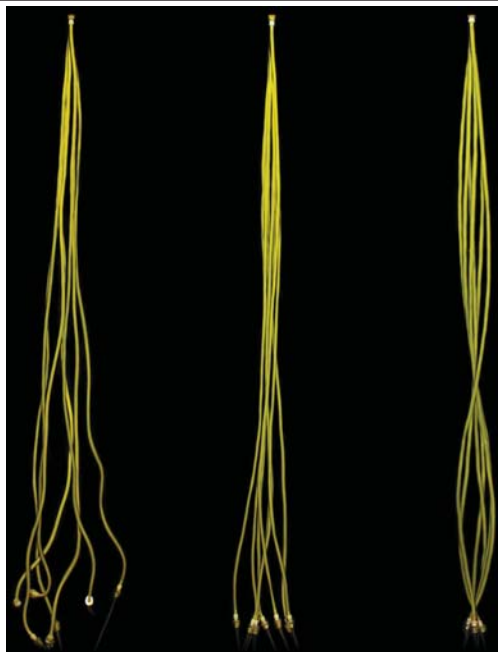
Figure 5.8 Composite photographs of 3 tubes and rotational stabilization. The left image shows no forced rotation, the middle image shows some stabilization after forced rotation, and the right image shows rigid rotation at a critical rotation speed.
