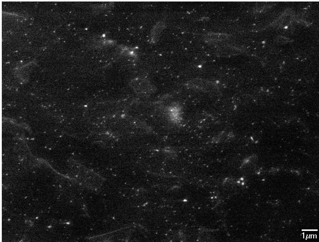
Figure A-12 BSE-SEM image of precipitates from X80-B4F steel.
