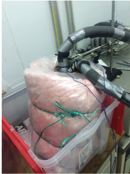
FIGURE B.25 Power loss test, fiberglass insulation (the copper coil was cover complete).
