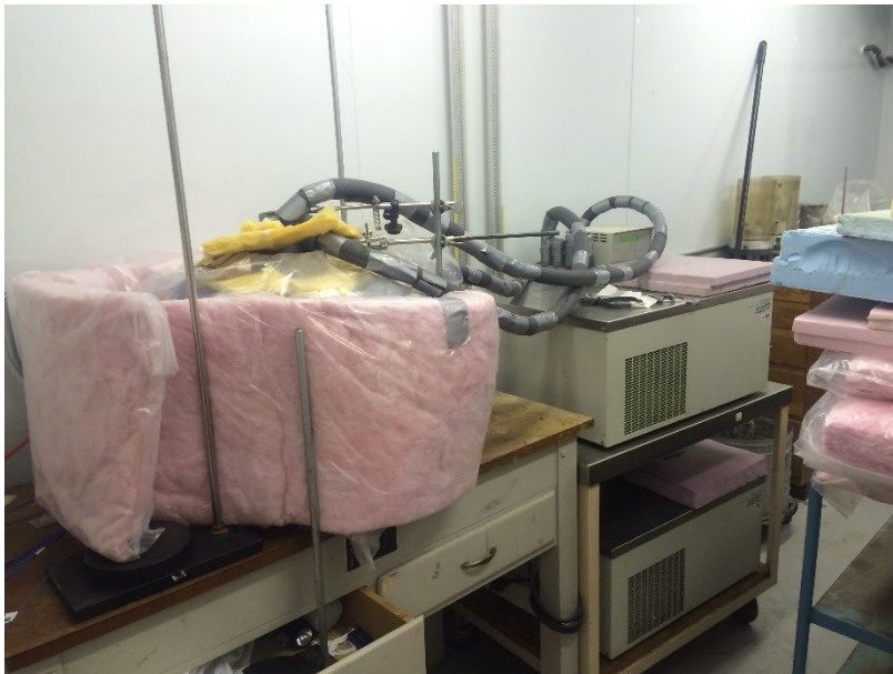
FIGURE B.22 Test cell fiberglass insulation (the test cell was cover complete) and hoses foam insulation.
