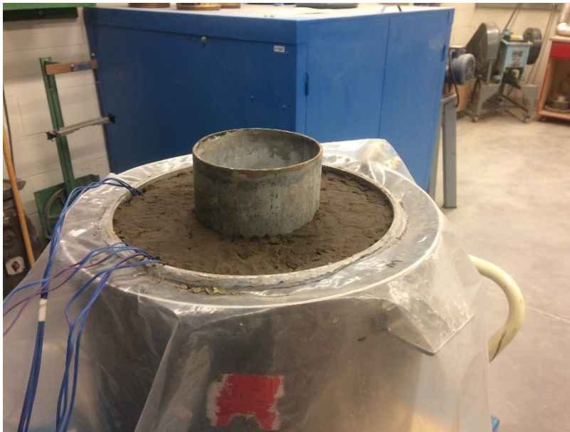
FIGURE B.18 Soil sample preparation w (20%).
