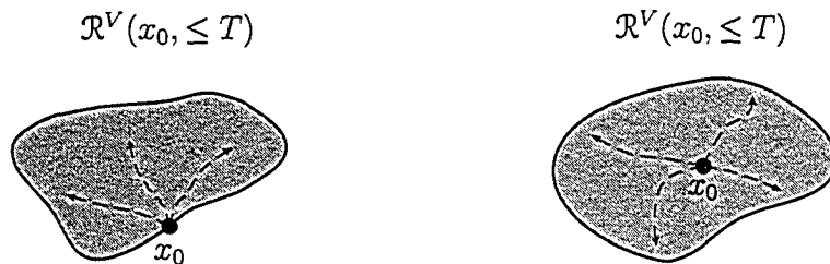
Figure. 2.1: Illustration of a system accessible from x_0 (left) and STLC from x_0 (right).
