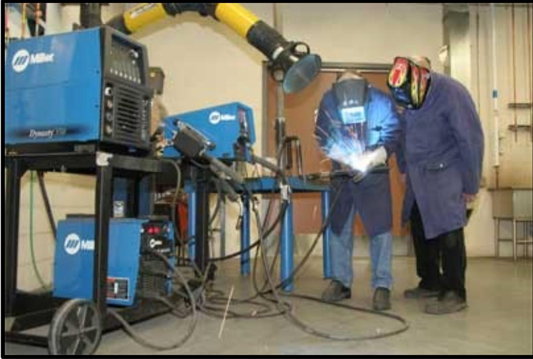
*Figure 1.1 The local exhaust ventilation system at NAIT Souch Campus. A standard in all welding labs at NAIT, Souch Campus. [52].*
