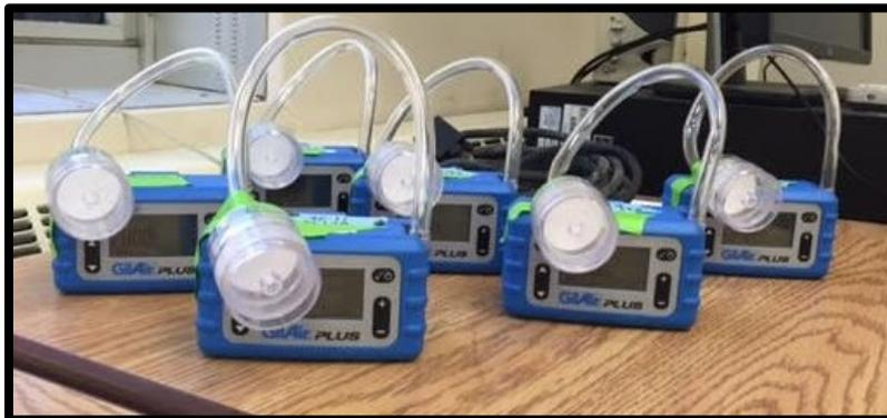
Figure 2.3 Ambient and personal air sampling set-up. Representations of the placement and arrangement of the air sampling pumps for ambient (a) and personal (b) sampling. As seen in the diagram, the cassette was attached to the collar of the welders, in the personal breathing zone, the tubing would have looped under the welding jacket. The picture presented in (c) represents the pumps used and how they would have been set-up for ambient air collection.
