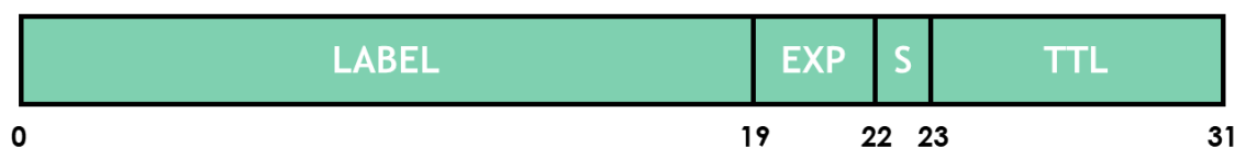
Figure 3-1: Segment ID in MPLS Data Plane [1]
