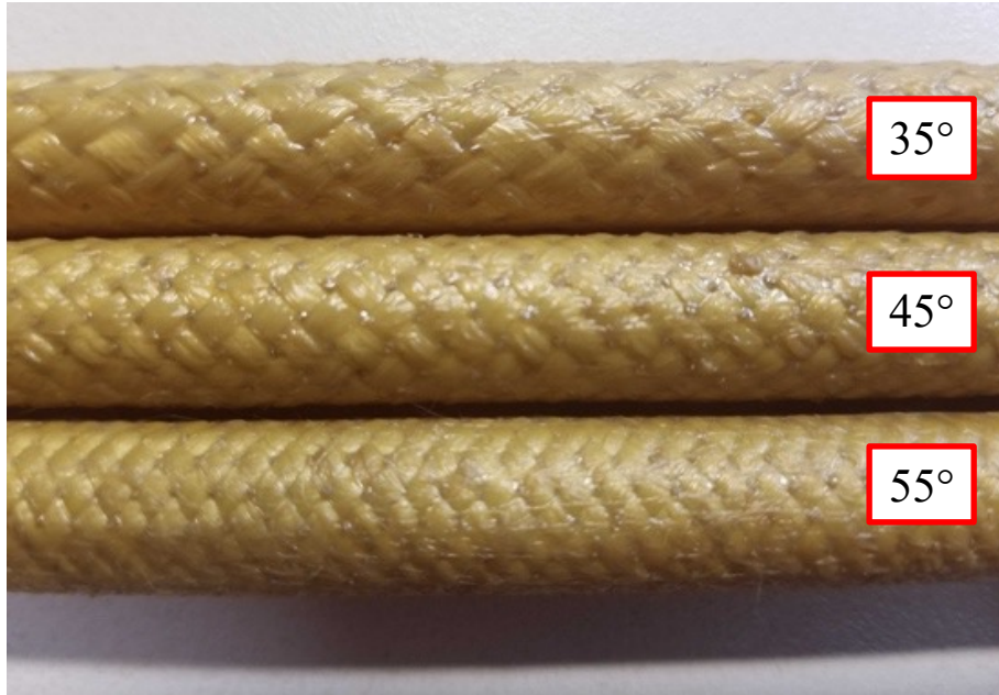
Figure 4.8. Kevlar/epoxy TBC samples manufactured at the three braid angles used in this work, 35°, 45° and 55°.
