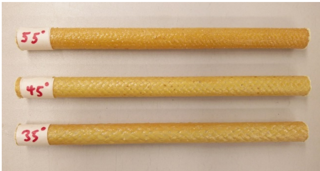
Figure 6.5. Cured TBC samples manufactured at three braid angles, 35, 45 and 55 degrees.
