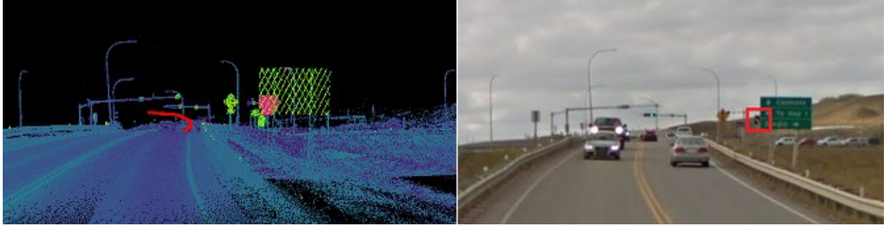
Figure 67 Sign 37 occluded by sign 36 in the point cloud data (left) and a picture of the road (right)
