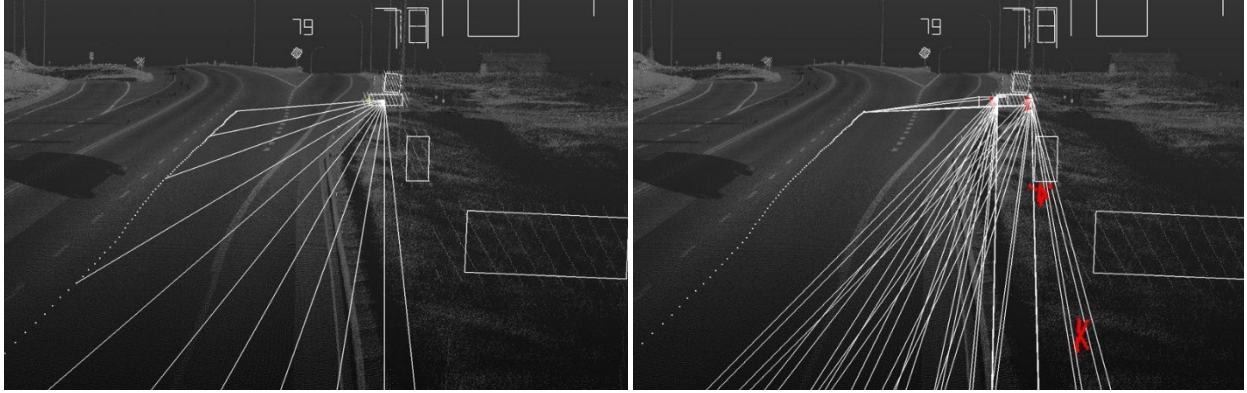
Figure 59 Sign c_{77} \in C obstructions
