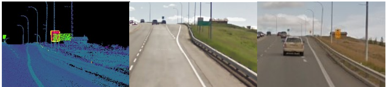
Figure 63 A comparison for the location of signs 77 and 78. On the left, the point cloud data. In the middle, an image of the location before the change. On the right, the same location after sign 77 was removed
