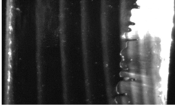
Figure 6.13 – A 0.5% solids solution of  $\sim 48$  nm diameter Orange (540 Ex/560 Em) FluoSpheres mixed with optical adhesive, with the water evaporated, was inserted into the wide end of a taper (at right). The result is a much more uniform distribution of microspheres suspended in optical adhesive. The evaporation of the water also helped to increase the viscosity of the mixture, preventing the mixture from infiltrating too far into the taper cavity before being cured.
