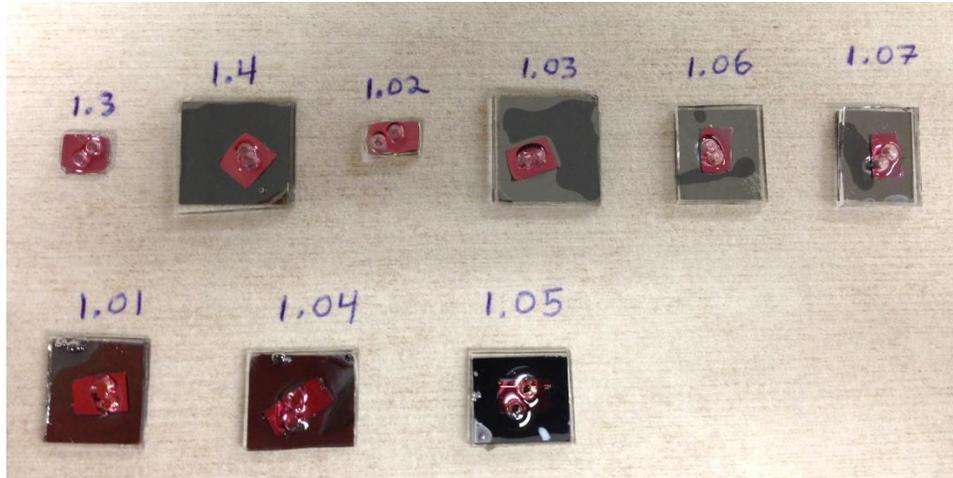
Figure 4.4 – Photo of hollow waveguide samples with PDMS wells fabricated on top. Partial delamination of non-essential areas is visible for samples 1.03, 1.06, and 1.07. The addition of an oxygen plasma step during fabrication eliminated this problem, shown in samples 1.01, 1.04, and 1.05.
