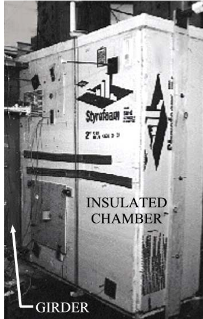
Figure 3–11 West Side of Insulated Chamber Surrounding Joint 10, Specimen 1
