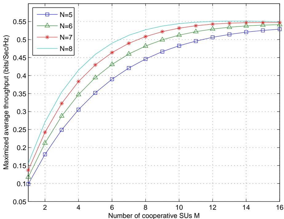
Figure 4.13. The SUs' maximized average throughput versus  $M$ , for different values of  $N$ , with  $\mu_1 = 0.5$ ,  $\frac{Y_{th}}{\sigma^2} = 1.05$ .
