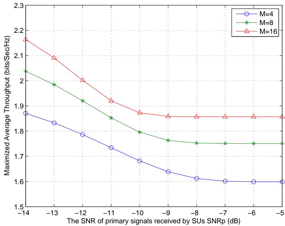
Figure 3.4. The maximized average throughput of the SUs versus  $\text{SNR}_p$  for different numbers of SUs,  $M$ , with  $\frac{Y_{th}}{\sigma^2} = 1.05$ .
