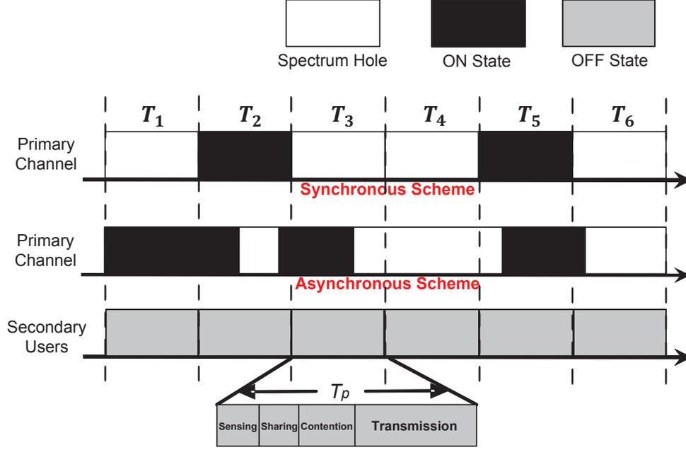
Figure 4.3. Comparison between the traditional synchronous schemes and the proposed asynchronous scheme.
