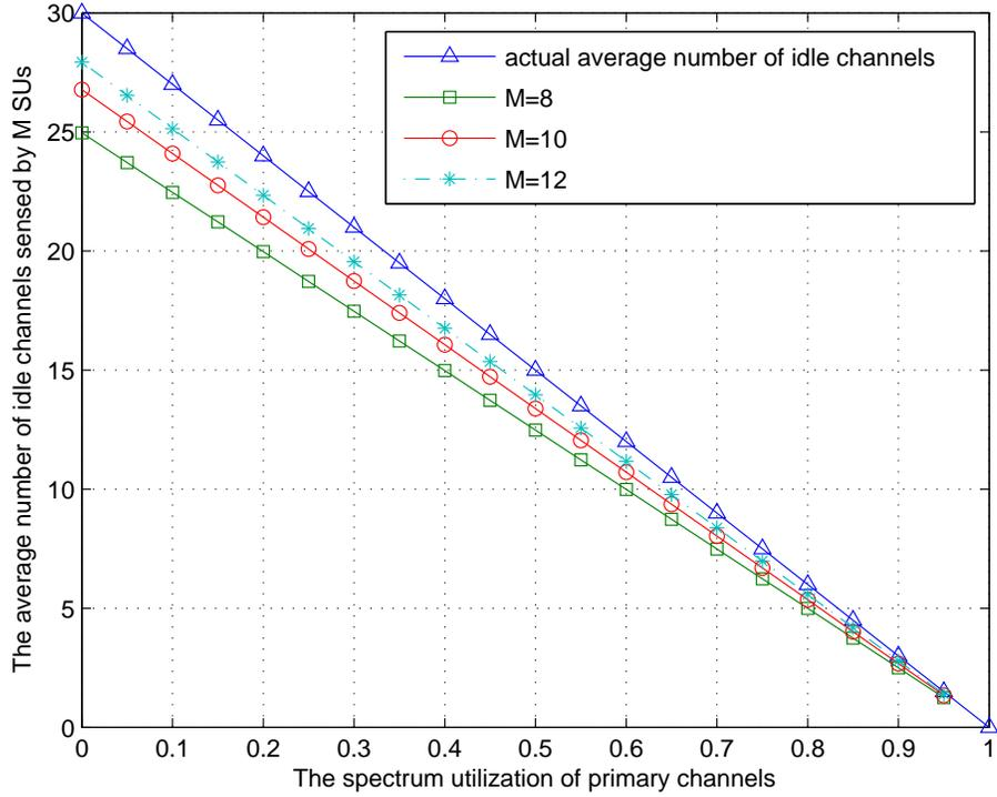
Figure 4.11. The average number of idle channels sensed by different numbers of cooperative SUs,  $M$ , when  $N = 6$  channels are sensed by one SU.
