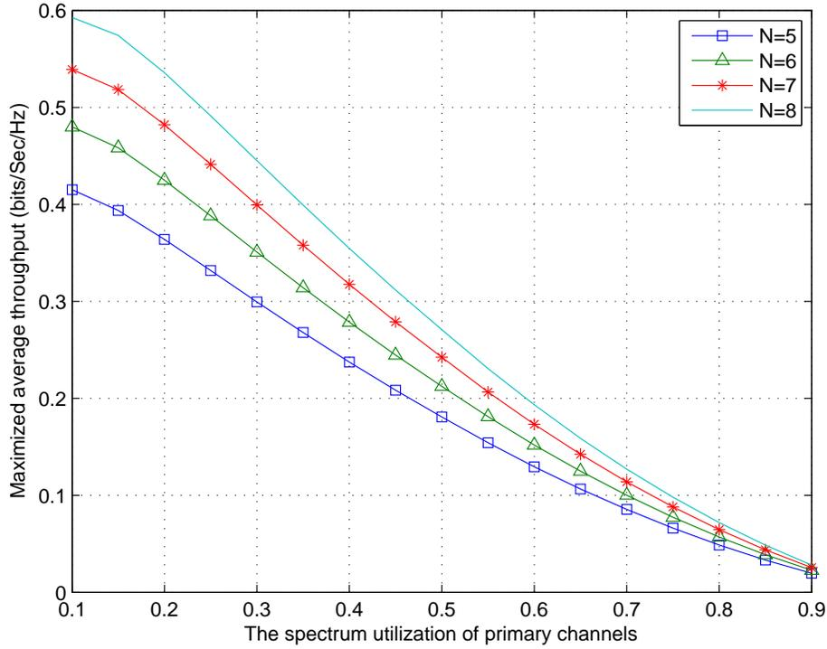
Figure 4.12. The maximized average throughput of  $M = 2$  SUs versus  $\mu_1$ , for different values of  $N$ , with  $\frac{Y_{th}}{\sigma^2} = 1.05$ .
