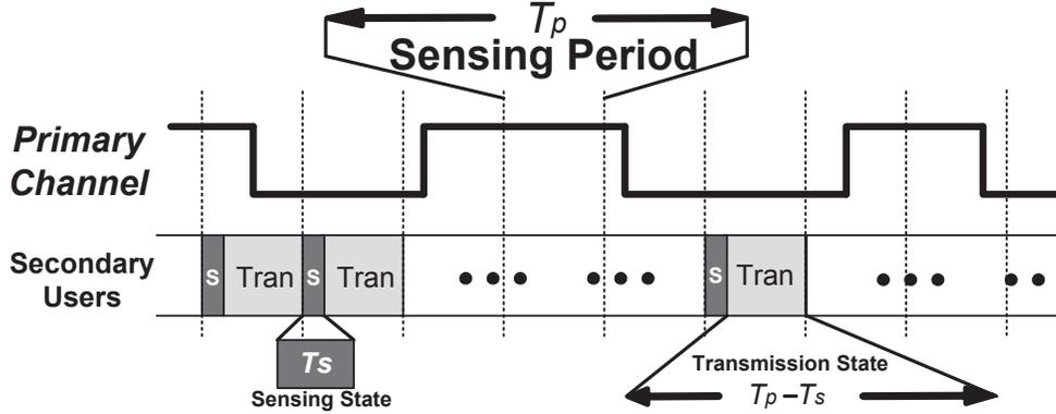
Figure 3.1. The asynchronous cooperative spectrum sensing scheme.
