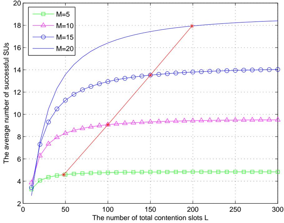
Figure 4.8. The average number of successful SUs versus the number of total contention slots,  $L$ , for different numbers of SUs,  $M$ . The straight line gives the quiescent points for different values of  $M$ .
