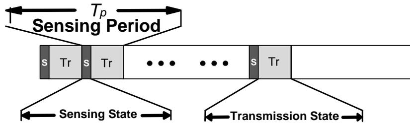
Figure 2.3. The frame structure of periodic spectrum sensing.
