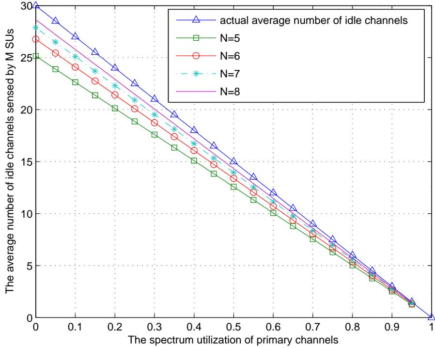
Figure 4.10. The average number of idle channels sensed by  $M = 10$  SUs for different numbers of primary channels sensed by one SU,  $N$ .
