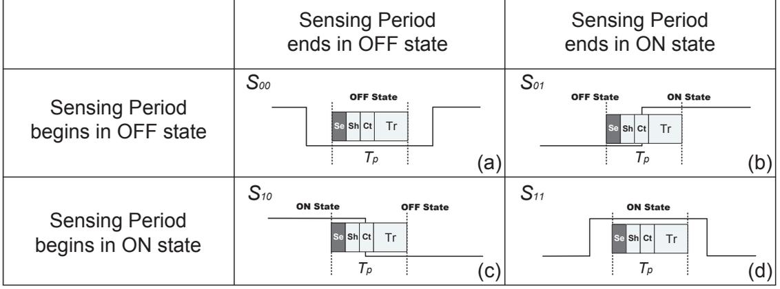
Figure 4.9. Four different cases of asynchronism between SUs and PUs.
