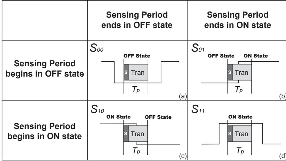
Figure 3.2. Four different cases of asynchronism between SUs and PU.
