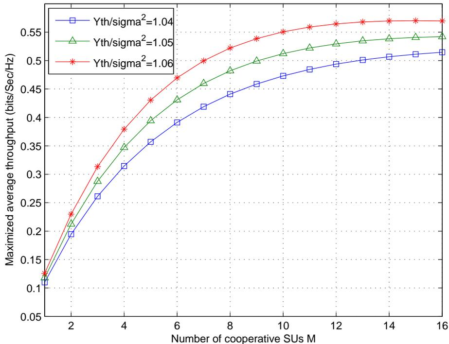
Figure 4.14. The SUs' maximized average throughput versus  $M$ , for different values of  $\frac{Y_{th}}{\sigma^2}$ , with  $\mu_1 = 0.5$ ,  $N = 6$ .
