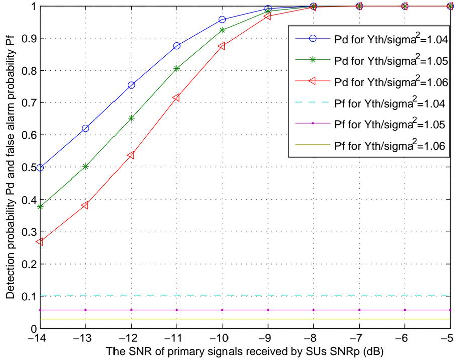
Figure 3.3. The detection probability and false alarm probability versus  $\text{SNR}_p$  for different decision thresholds with  $M = 10$ .
