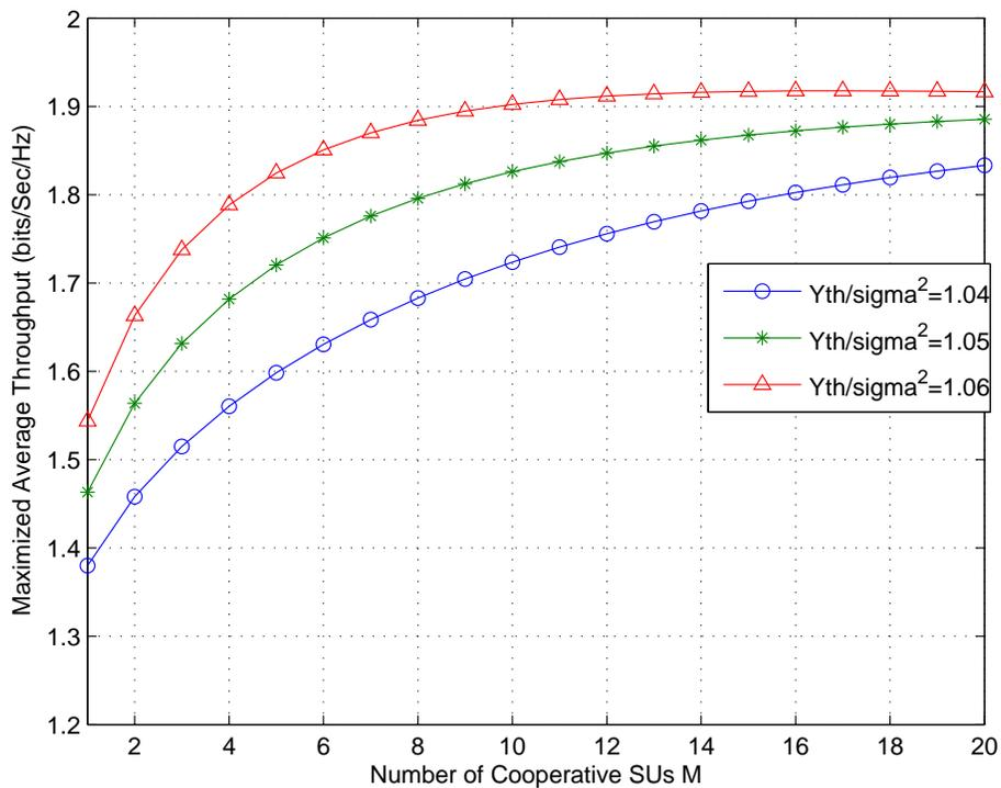
Figure 3.5. The maximized average throughput of the SUs versus  $M$  for different values of  $\frac{Y_{th}}{\sigma^2}$  with  $\text{SNR}_p = -10$  dB.
