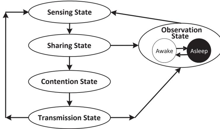
Figure 4.2. The SUs' state transition diagram.
