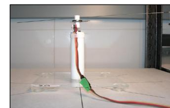
Figure 9: Flight mill apparatus
